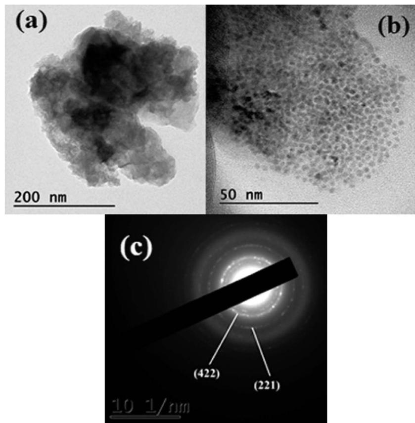
Fig. 4 TEM and HRTEM images of CoMnNiS sample (a) high and (b) low resolution (c) SAED pattern showing various diffraction planes, *i.e.* (221) of NiS<sub>2</sub> and (422) of MnS<sub>2</sub>.
