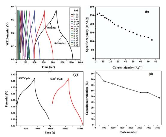
Fig. 7 Galvanostatic charge–discharge of CoMnNiS electrode (a) GCD profiles at various current densities (b) plot of specific capacitance vs. current densities  $(2.5-75 \text{ A g}^{-1})$  (c) cyclic stability curve at different cycles at 50 A g<sup>-1</sup> (d) plot of capacitance retention vs. no. of cycles at 50 A g<sup>-1</sup>.
