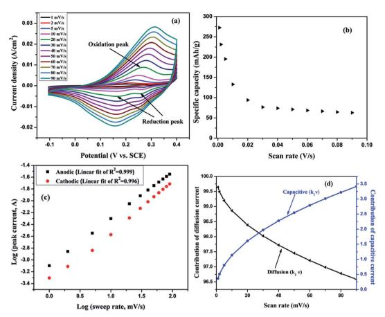
Fig. 6 Cyclic voltammetry of CoMnNiS electrode (a) CV curve at various scan rates in the range 1–90 mV s<sup>-1</sup> showing oxidation and reduction peaks, (b) plot of variation of specific capacitance vs. scan rate  $(1-90 \text{ mV s}^{-1})$ , (c) plot of log(peak current, A) vs. log(sweep rate, mV s<sup>-1</sup>) showing linear behavior (d) plot of variation of diffusion and capacitive current vs. scan rate.
