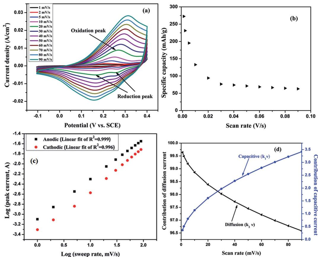
Fig. 6 Cyclic voltammetry of CoMnNiS electrode (a) CV curve at various scan rates in the range 1–90 mV s<sup>-1</sup> showing oxidation and reduction peaks, (b) plot of variation of specific capacitance vs. scan rate (1–90 mV s<sup>-1</sup>), (c) plot of log(peak current, A) vs. log(sweep rate, mV s<sup>-1</sup>) showing linear behavior (d) plot of variation of diffusion and capacitive current vs. scan rate.
