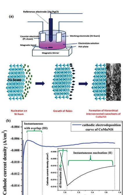
Fig. 1 (a) Experimental arrangement for electrodeposition and schematic representation of CoMnNiS formation on Ni foam (b) cathodic electrodeposition curve of 10 min duration (chronoamperometry), indicating various processes taking place during deposition of CoMnNiS on Ni foam; (inset) magnified image of region I & II of the chronoamperometry curve.
