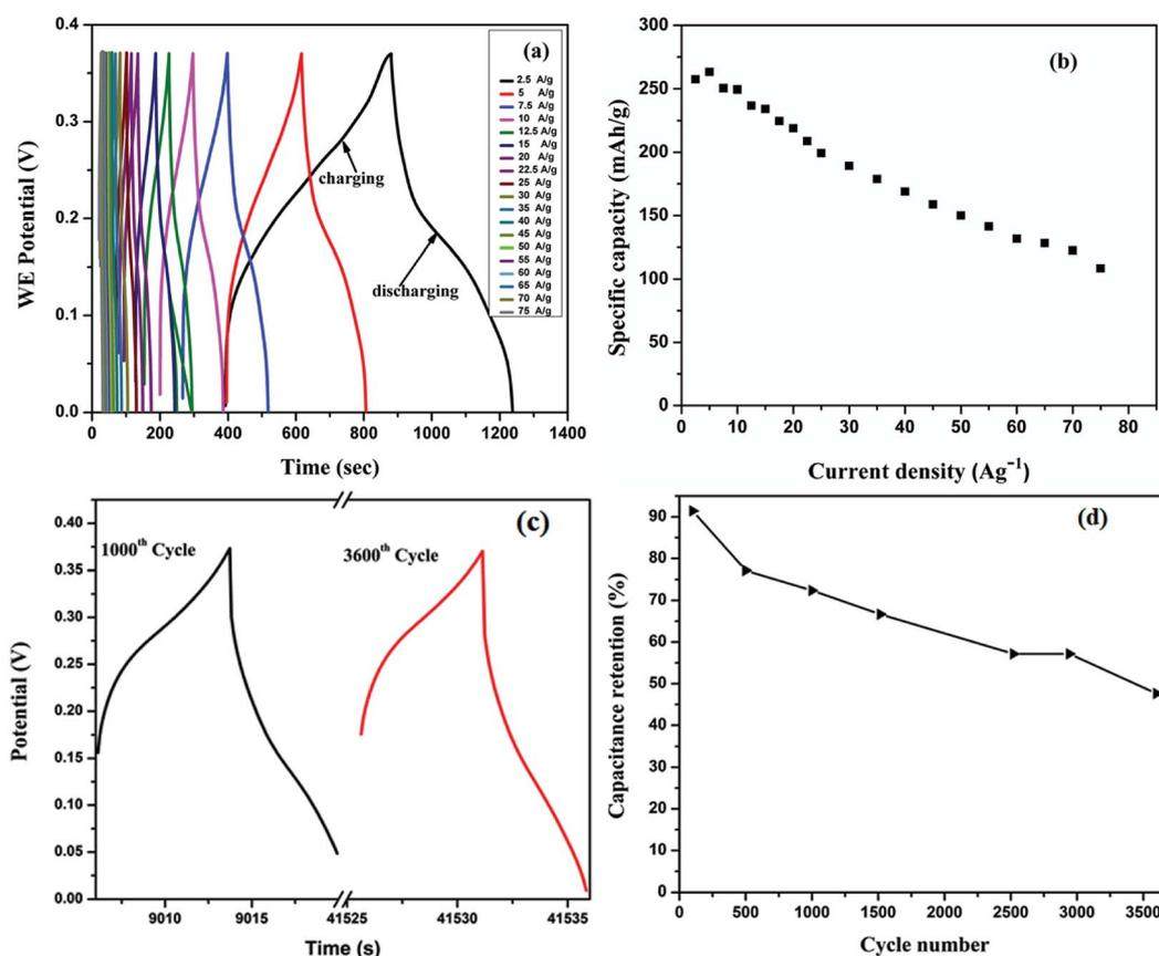
Fig. 7 Galvanostatic charge–discharge of CoMnNiS electrode (a) GCD profiles at various current densities (b) plot of specific capacitance vs. current densities ( $2.5\text{--}75\text{ A g}^{-1}$ ) (c) cyclic stability curve at different cycles at  $50\text{ A g}^{-1}$  (d) plot of capacitance retention vs. no. of cycles at  $50\text{ A g}^{-1}$ .
