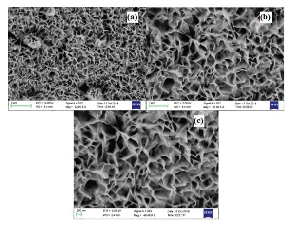
Fig. 3 FESEM images (a-c) of CoMnNiS sample showing hierarchical interconnected nanosheets-like morphology at different magnifications (2 um to 200 nm).
