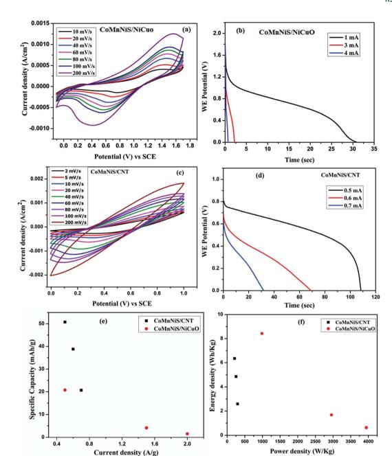
Fig. 9 Asymmetric device (a) cyclic voltammogram and (b) discharge curves, at different scan rates and current for CoMnNiS/NiCuO (c) cyclic voltammogram and (d) discharge curves, at different scan rates and current for CoMnNiS/CNT. Comparison of the variation of (e) specific capacity with current density (f) energy density with power density (Ragone plot) of both the nanomaterials.
