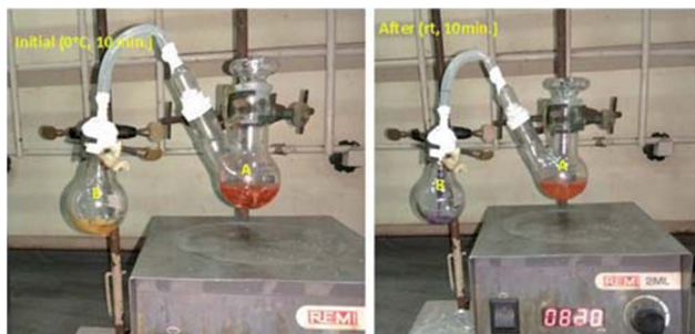
Fig. 3 Mechanistic study (ammonia trapping experiments).
