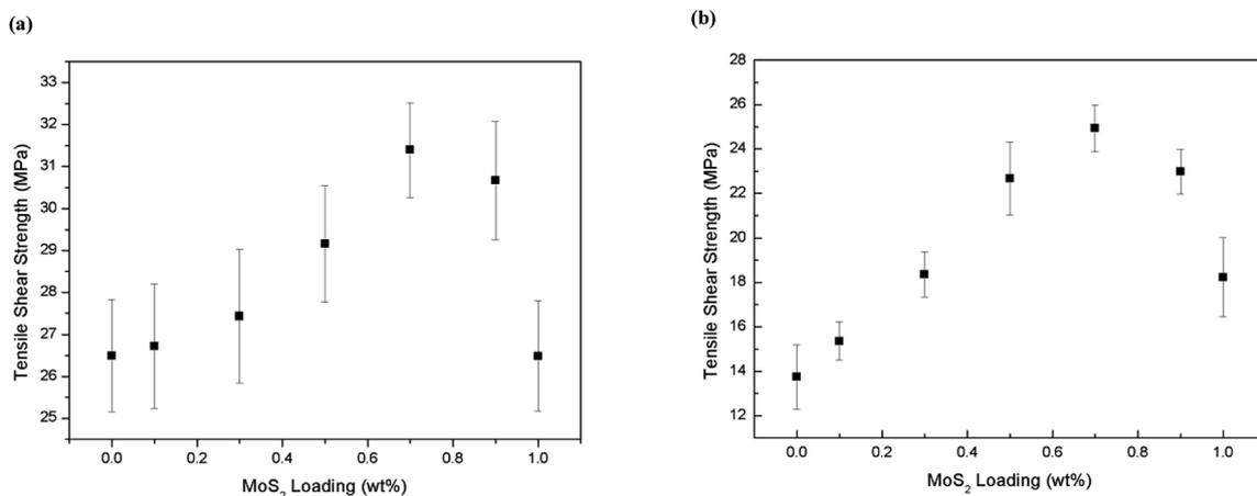
Fig. 5 (a) Apparent shear strength at room temperature vs. f-MoS<sub>2</sub> nanosheets loading fraction; (b) apparent shear strength at 120 °C vs. f-MoS<sub>2</sub> nanosheets loading fraction.
