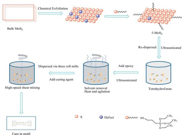
Scheme 1 Schematic illustration of f-MoS<sub>2</sub>/epoxy composite preparation route.
