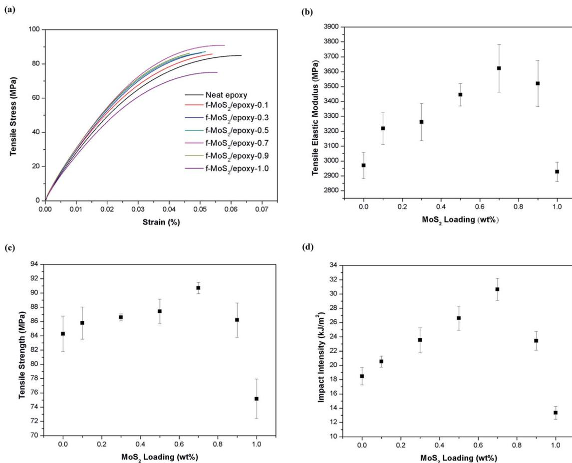
Fig. 4 (a) Stress–strain curves of neat epoxy and f-MoS<sub>2</sub>/epoxy nanocomposites with various loadings of f-MoS<sub>2</sub>; (b) Young's modulus vs. f-MoS<sub>2</sub> nanosheets loading fraction; (c) ultimate tensile strength vs. f-MoS<sub>2</sub> nanosheets loading fraction; (d) impact intensity vs. f-MoS<sub>2</sub> nanosheets loading fraction.
