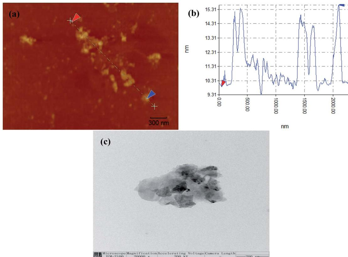
Fig. 1 AFM images (a) and thickness profiles (b) of f-MoS<sub>2</sub> nanosheets; TEM images of f-MoS<sub>2</sub> (c).
