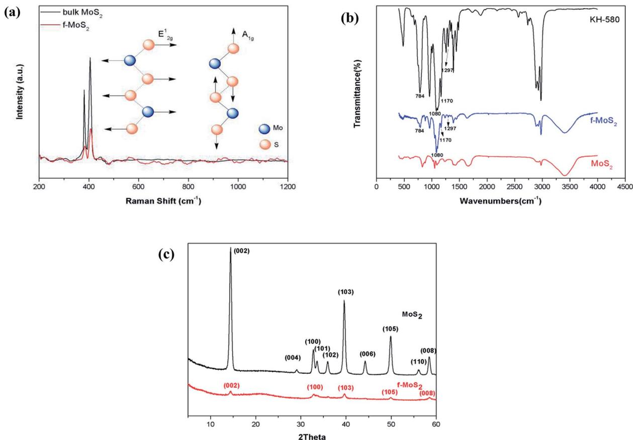
Fig. 2 (a) Raman spectrum of bulk MoS<sub>2</sub> and f-MoS<sub>2</sub> nanosheets; (b) Fourier transform infrared spectra of KH580, MoS<sub>2</sub> and f-MoS<sub>2</sub>; (c) Powder X-ray diffraction patterns of MoS<sub>2</sub> and f-MoS<sub>2</sub>.
