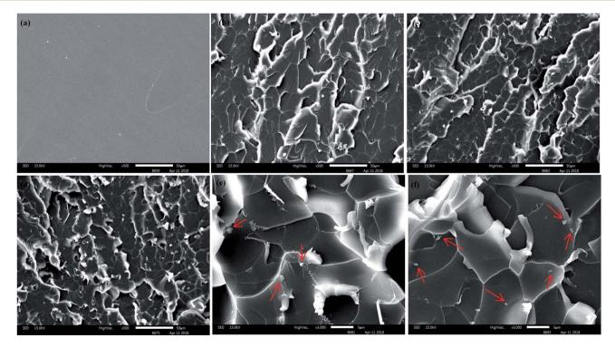
Fig. 6 Scanning electron microscopy images of the fracture surfaces of neat EP (a),  $0.3 \text{ wt\% f-MoS}_2/\text{epoxy}$  (b),  $0.7 \text{ wt\% f-MoS}_2/\text{epoxy}$  (c and e) and  $1.0 \text{ wt\% f-MoS}_2/\text{epoxy}$  (d and f) nanocomposites.
