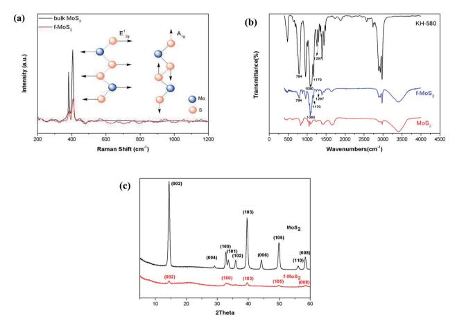
Fig. 2 (a) Raman spectrum of bulk  $MoS_2$  and  $f-MoS_2$  nanosheets; (b) Fourier transform infrared spectra of KH580,  $MoS_2$  and  $f-MoS_2$ ; (c) Powder X-ray diffraction patterns of  $MoS_2$  and  $f-MoS_2$ .
