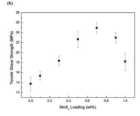
Fig. 5 (a) Apparent shear strength at room temperature vs. f-MoS<sub>2</sub> nanosheets loading fraction; (b) apparent shear strength at 120 °C vs. f-MoS<sub>2</sub> nanosheets loading fraction.
