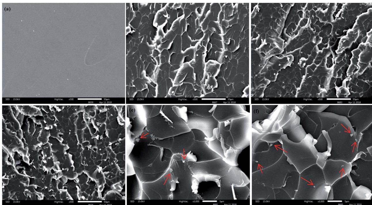
Fig. 6 Scanning electron microscopy images of the fracture surfaces of neat EP (a), 0.3 wt% f-MoS<sub>2</sub>/epoxy (b), 0.7 wt% f-MoS<sub>2</sub>/epoxy (c and e) and 1.0 wt% f-MoS<sub>2</sub>/epoxy (d and f) nanocomposites.
