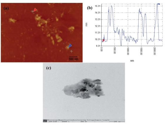
Fig. 1 AFM images (a) and thickness profiles (b) of f-MoS<sub>2</sub> nanosheets; TEM images of f-MoS<sub>2</sub> (c).
