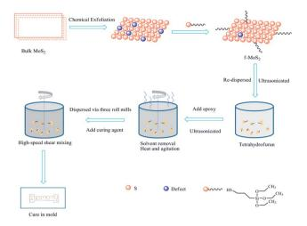
Scheme 1 Schematic illustration of  $f\text{-MoS}_2$ /epoxy composite preparation route.
