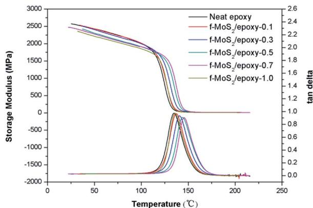
Fig. 3 Plots of storage modulus and tan delta versus temperature for neat epoxy and f-MoS<sub>2</sub>/epoxy composites.
