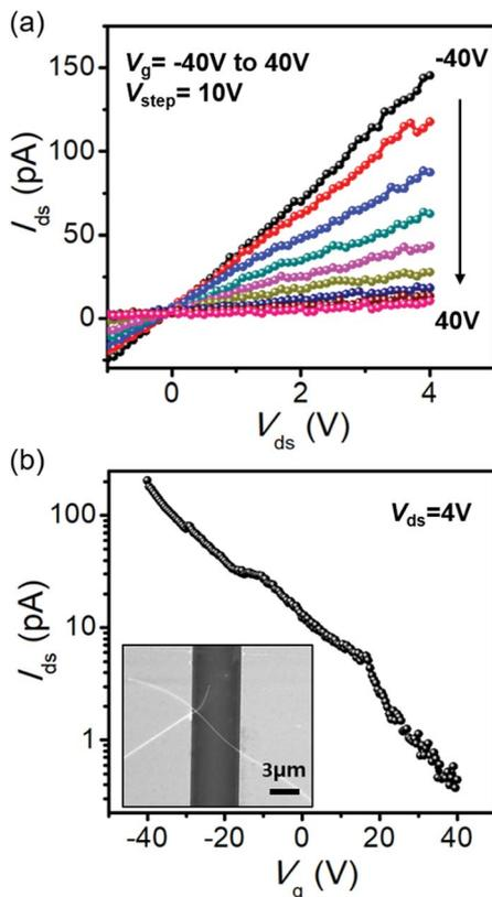
Fig. 6 (a) Current–voltage ( $I_{ds}$ – $V_{ds}$ ) characteristics of the  $Nb_2Se_9$  FET. (b) Transfer characteristics ( $I_{ds}$ – $V_g$ ) of the  $Nb_2Se_9$  FET.  $V_g = -40$  V to 40 V. Inset shows SEM image of the  $Nb_2Se_9$  FET.
