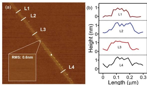
Fig. 4 AFM image of exfoliated quasi-two-dimensional monolayer Nb<sub>2</sub>Se<sub>9</sub> on 300 nm SiO<sub>2</sub>/Si substrate. The inset shows the HR-AFM image of selected regions and its RMS value. (b) Line profile of quasi-two-dimensional monolayer Nb<sub>2</sub>Se<sub>9</sub> ribbon as marked L1, L2, L3, and L4 in (a).
