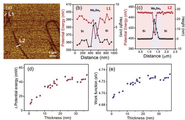
Fig. 5 (a) SKPM image of the exfoliated Nb<sub>2</sub>Se<sub>9</sub> flakes on an Si substrate; (b) and (c) height and potential energy profiles of the Nb<sub>2</sub>Se<sub>9</sub> flakes and Si substrate, as marked in (a); (d) and (e) variation of the potential energy difference and work function according to the thickness of the Nb<sub>2</sub>Se<sub>9</sub> flakes.
