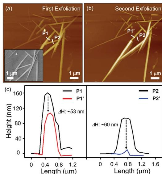
Fig. 3 (a) AFM image of the exfoliated quasi-two-dimensional Nb<sub>2</sub>Se<sub>9</sub> flakes on a 300 nm SiO<sub>2</sub>/Si substrate. (b) AFM image of the exfoliated Nb<sub>2</sub>Se<sub>9</sub> flakes on a 300 nm SiO<sub>2</sub>/Si substrate after an additional peeling process. (c) Line profile of the Nb<sub>2</sub>Se<sub>9</sub> flakes before and after a second exfoliation.
