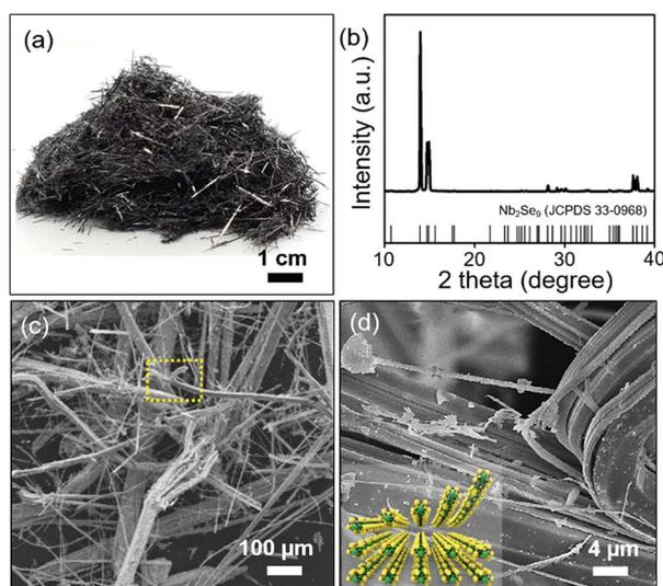
Fig. 1 (a) Photograph of the mass-production of needle-like  $\text{Nb}_2\text{Se}_9$  crystals; (b) XRD pattern of the  $\text{Nb}_2\text{Se}_9$  crystal; (c) and (d) low- and high-magnification SEM images of the  $\text{Nb}_2\text{Se}_9$  crystal. The inset shows an illustration of the crystal structure of  $\text{Nb}_2\text{Se}_9$ .
