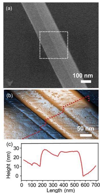
Fig. 2 (a) SEM and (b) 3D AFM images of the exfoliated quasi-two-dimensional  $\text{Nb}_2\text{Se}_9$  flake on a 300 nm  $\text{SiO}_2/\text{Si}$  substrate. (c) Line profile of the corresponding  $\text{Nb}_2\text{Se}_9$  flakes, as marked in (b).
