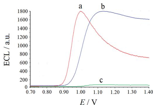
Fig. 3 ECL responses of  $2.0 \times 10^{-4}$  mmol  $\text{mL}^{-1}$   $\text{Ru}(\text{bpy})_3^{2+}$  solution in the presence of  $4.0 \times 10^{-4}$   $\mu\text{mol mL}^{-1}$  TPRA (a),  $6.8 \times 10^{-9}$   $\mu\text{mol mL}^{-1}$  AuNPs (b) and absence (c).
