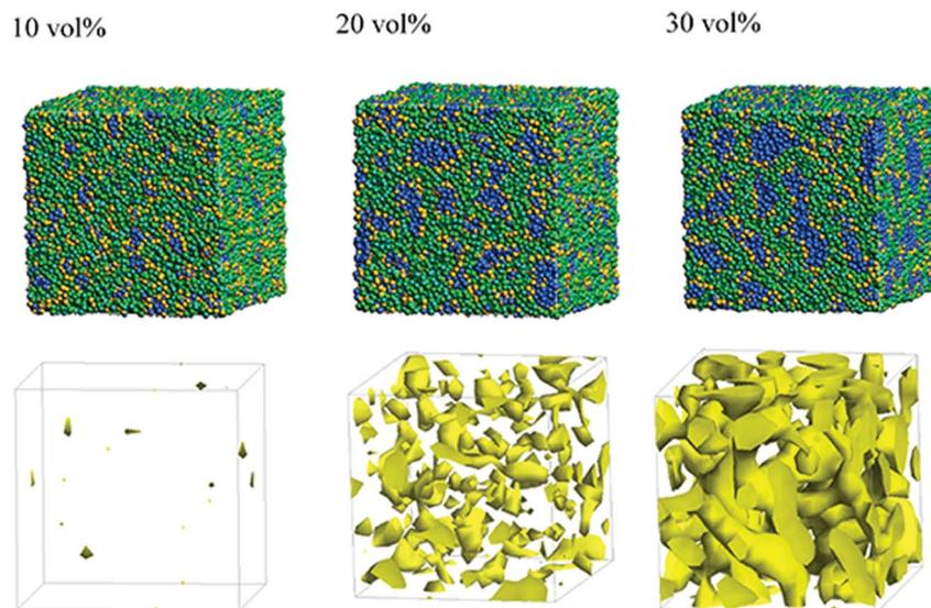
Fig. 9 Dependence of morphology on water contents for SPEEK ( $t = 500$ ). Morphologies of 10, 20, and 30 vol% are depicted in upper row. Water density distributions are given drawn in lower row.
