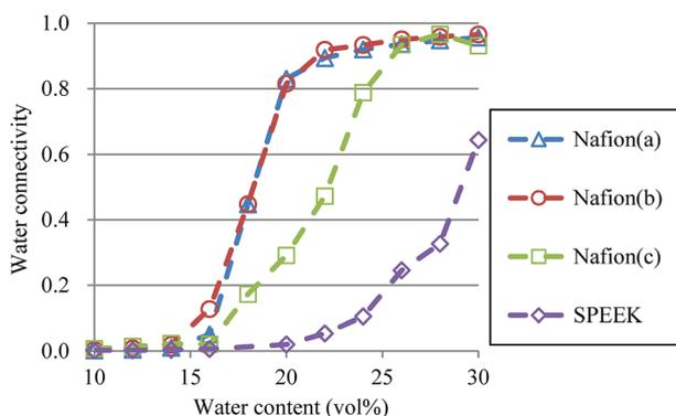
Fig. 14 Water connectivity plots for Nafion and SPEEK with respect to water contents using the transient structure of every 100 steps. Symbols of triangle, circle, and square represent the results of symbolic structures (a), (b), and (c) of Nafion in Fig. 4, respectively. Symbol of diamond corresponds to SPEEK.
