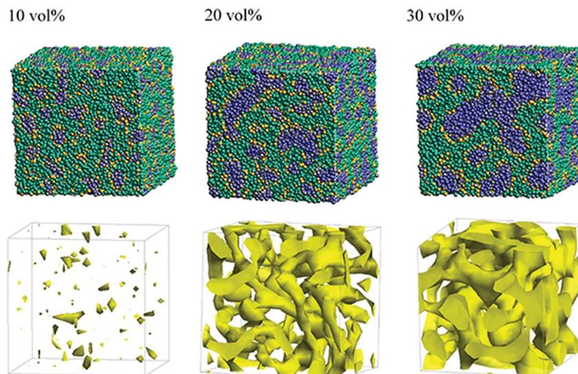
Fig. 8 Dependence of morphology on water contents for Nafion ( $t = 500$ ) with symbolic structure (b) in Fig. 4. Morphologies of 10, 20, and 30 vol% are depicted in upper row. Water density distributions are given drawn in lower row.
