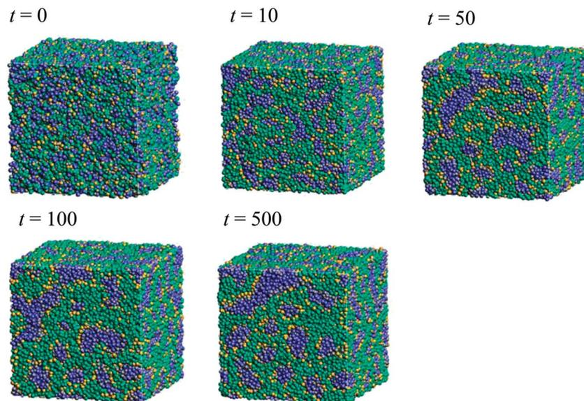
Fig. 5 Time-dependent (with symbol "t") morphologies of the case of 20 vol% water content for Nafion with symbolic structure (b) shown in Fig. 4. Hydrophobic, hydrophilic, and water particles are depicted with green, yellow and blue colors, respectively.
