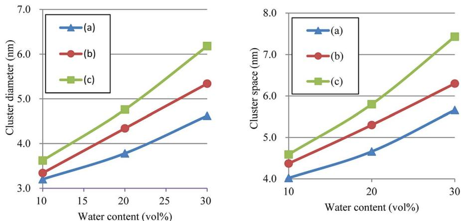
Fig. 12 Dependences of cluster diameter and space on water contents of 10, 20 and 30 vol% for Nafion. Symbols of triangle, circle and square represent the results of symbolic structures (a), (b) and (c) in Fig. 4.
