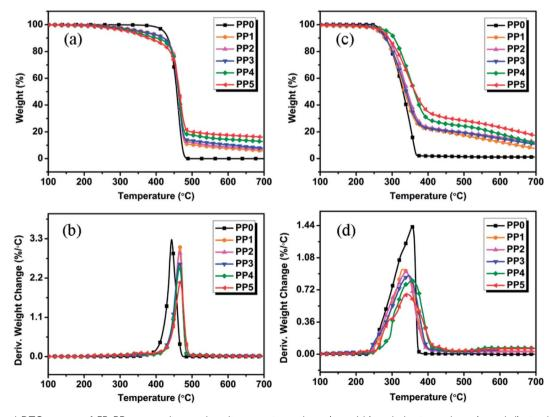
Fig. 3 TGA and DTG curves of FR PP composites under nitrogen atmosphere (a and b) and air atmosphere (c and d) at a heating rate of  $10 \, ^{\circ}$ C min $^{-1}$ .
