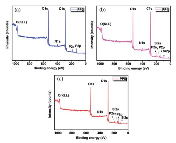
The XPS survey spectra of char residue of PP2 (a), PP4 (b) and PP5 (c) after UL94 vertical burning test.
