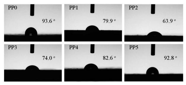
Fig. 10 The digital photos of water contact angle for different FR PP composites.
