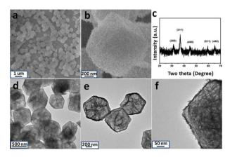
Fig. 2 SEM (a and b), TEM images (d to f) and XRD pattern (c) of Co<sub>3</sub>O<sub>4</sub>@NiCo<sub>2</sub>O<sub>4</sub> sheets-in-cage hybrid nanoparticle
