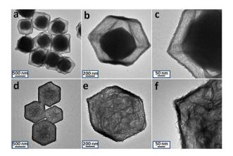
Fig. 1 TEM images of ZIF-67@NiCo-LDH yolk@shell nanoparticles (a to c) and Co(OH)<sub>2</sub>@NiCo-LDH sheets-in-cage nanoparticles (d to f).
