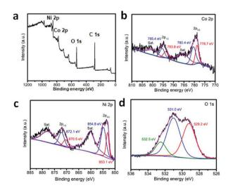
Fig. 3 XPS spectra of Co<sub>3</sub>O<sub>4</sub>@NiCo<sub>2</sub>O<sub>4</sub> sheets-in-cage hybrid nanoparticles.
