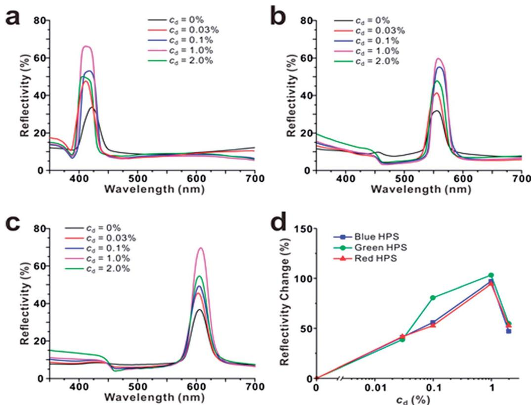
Fig. 4 (a–d) Reflectivity changes of (a) blue ( $d_{\text{SiO}_2} = 159 \pm 9$  nm), (b) green ( $d_{\text{SiO}_2} = 174 \pm 10$  nm) and (c) red HPSs ( $d_{\text{SiO}_2} = 199 \pm 9$  nm) with the increase of the PDA nanoparticle concentration ( $0 \leq c_d \leq 2.0$ ). The reflectivity increased logarithmically as a function of the dopant concentration with showing a maximum at  $c_d = 1.0\%$ .
