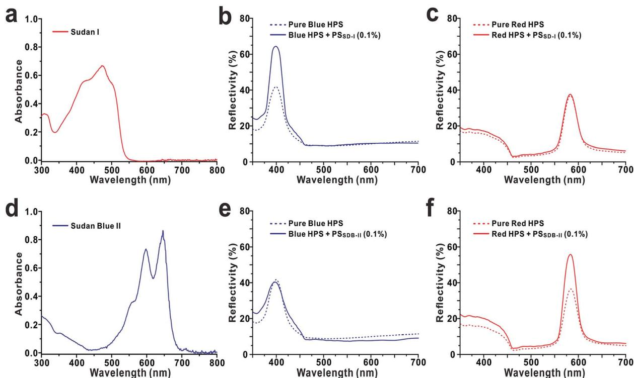
**Fig. 2** Absorbance spectra of (a) Sudan I ( $c = 0.05$  mM) and (d) Sudan Blue II ( $c = 0.05$  mM). Reflectivity changes of the blue HPSs ( $\lambda_{\text{peak}} = 400$  nm) with the addition of (b) PS<sub>SD-I</sub> and (e) PS<sub>SDB-II</sub>. Reflectivity changes of the red HPSs ( $\lambda_{\text{peak}} = 585$  nm) with the addition of (c) PS<sub>SD-I</sub> and (f) PS<sub>SDB-II</sub>.
