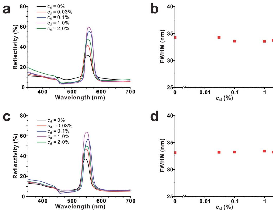
Fig. 5 (a and c) Reflectivity changes and (b and d) FWHM changes in green HPSs ( $d_{\text{SiO}_2} = 174 \pm 10 \text{ nm}$ ) with the addition of (a and b) size-matching ( $d_{\text{PDA}} = 172 \pm 16 \text{ nm}$ ) and (c and d) size-mismatching PDA nanoparticles ( $d_{\text{PDA}} = 106 \pm 8 \text{ nm}$ ).
