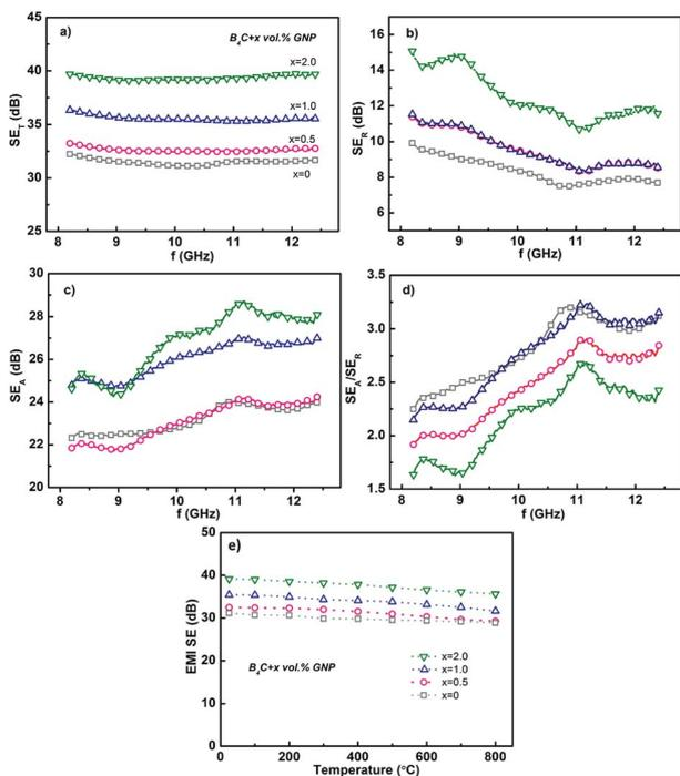
Fig. 4 (a)–(c) represent the frequency dependencies of  $SE_T$ ,  $SE_R$  and  $SE_A$  respectively of GNP/ $B_4C$  composites at room temperature; (d) frequency dependency of  $SE_A/SE_R$ ; (e) temperature dependency of  $SE_T$  for GNP/ $B_4C$  composites with different GNP loading.
