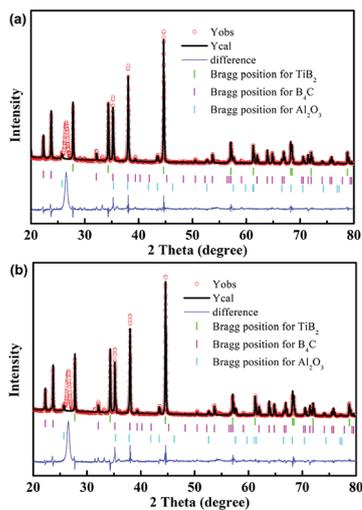
Fig. 1 Typical XRD patterns and XRD refinements of GNP/B<sub>4</sub>C composites with (a) 0 vol% and (b) 2 vol% GNPs.
