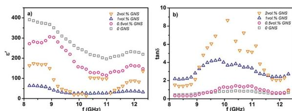
Fig. 6 (a) The real permittivity and (b) the dielectric loss of various GNP/B<sub>4</sub>C composites.
