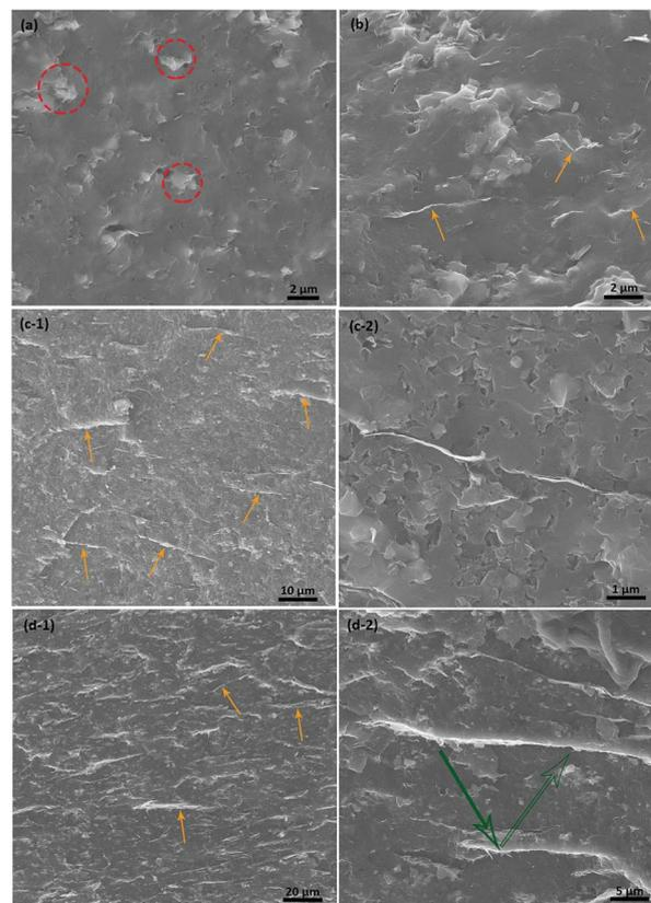
Fig. 2 Fracture surfaces of GNP/B<sub>4</sub>C composites with different GNP loading. (a) 0 vol%; (b) 0.5 vol%; (c-1) and (c-2) 1 vol%; (d-1) and (d-2) 2 vol%.
