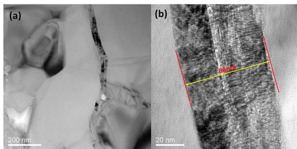
Fig. 3 TEM images of  $B_4C$ /GNP composites with 2 vol% GNPs. (a) Lower magnification; (b) higher magnification.
