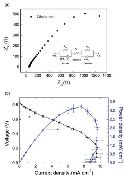
Fig. 4 (a) Nyquist plot of the LFMFC. The equivalent circuit model is shown in the inset. The Warburg impedance describes the diffusion resistance at anode ( $R_d$ ). CPE is the constant phase element related to the double layer capacitance. The subscripts a and c stand for anode and cathode, respectively. (b) The polarization and power density curves of the LFMFC.
