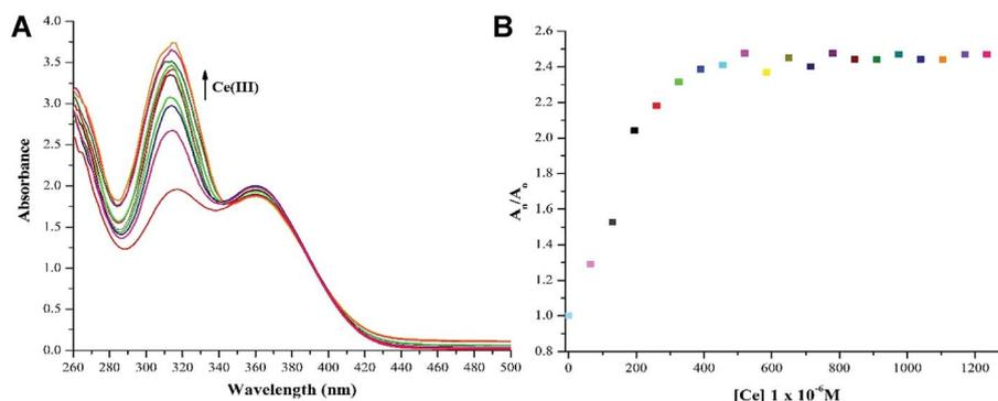
**Fig. 3** (a) 'Turn-on' response ( $\lambda_{\text{max}} = 322 \text{ nm}$ ) recorded with successive addition of  $60 \mu\text{M}$  solution of  $\text{Ce(III)}$  ions using DMSO as solvent owing to NTS– $\text{Ce(III)}$  ion interactions; (b) relative change in absorption maxima ( $A_n/A_o$ ) with addition of 15 equiv. of  $20 \mu\text{M}$  of  $\text{Ce(III)}$  ions; ( $A_o$  = absorption maxima of NTS;  $A_n$  = absorption maxima with successive addition of  $\text{Ce(III)}$  ions).
