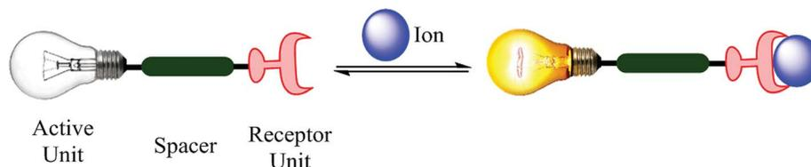
Fig. 1 Representation of a fluorescent ion luminescent sensor.
