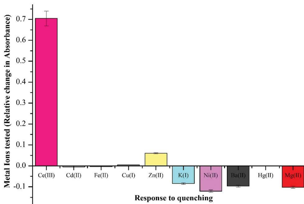
**Fig. 2** Competitive absorbance response recorded by luminescent sensor NTS with different cationic species using DMSO :  $\text{H}_2\text{O}$  4 : 1 (v/v) by addition of 5 equiv. of 20  $\mu\text{M}$  metal ion solution with recorded change in maxima value at  $\lambda = 322$  nm.
