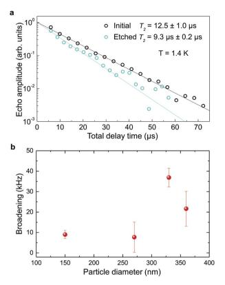
Fig. 7 Optical coherence lifetimes and homogeneous broadening. (a) Photon echo decays for initial and etched nanoparticles at 1.4 K with average sizes of 430 and 150 nm respectively.  $T_2$  values were derived by single exponential fit to the decay data. (b) Additional broadening due to etching as a function of the particles size. Error bars represent  $\pm 1$  standard deviation from several measurements.
