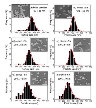
Fig. 1 Scanning electron microscopy (SEM) micrographs and size distributions of the initial and etched Eu<sup>3+</sup>:Y<sub>2</sub>O<sub>3</sub> nanoparticles for etching times increasing from 1 to 5 hours (etching temperature T = 50 °C)
