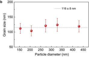
Fig. 3 XRD investigation. (a) Normalized diffraction peak for initial and etched particles with average sizes of 430 and 150 nm respectively. (b) Grain size as a function of particle size. The dotted line is a guide to the eye.
