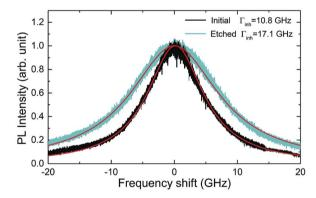
Fig. 6 Inhomogeneous broadening ( $\Gamma_{\rm inh}$ ) of the  $^7{\rm F_0} \rightarrow ^5{\rm D_0}$  optical transitions in initial (black) and etched (green) nanoparticles with average sizes of 450 and 200 nm respectively. Linewidths were estimated by Lorentzian fit.
