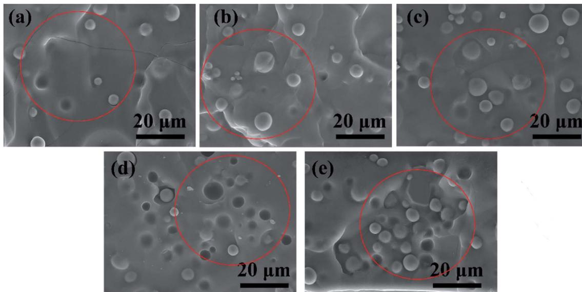
Fig. 9 Morphology evolution through-plane of PDMS/Al<sub>2</sub>O<sub>3</sub> (30 wt%) composites versus thickness: (a) thickness = 0.40 mm; (b) thickness = 0.30 mm; (c) thickness = 0.20 mm; (d) thickness = 0.15 mm; (e) thickness = 0.05 mm.
