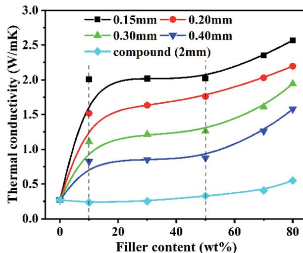
Fig. 5 Comparison of thermal conductivities of PDMS/Al<sub>2</sub>O<sub>3</sub> composites by SCFNA and compounding method.
