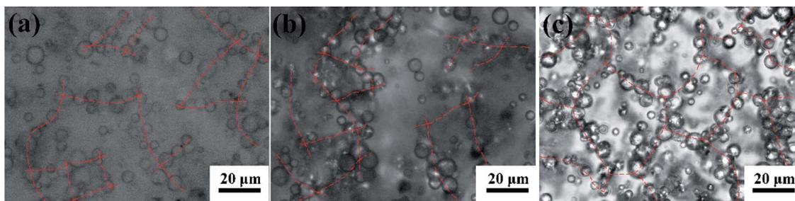
Fig. 8 Morphology evolution in-plane of PDMS/Al<sub>2</sub>O<sub>3</sub> (30 wt%) composites versus thickness: (a) thickness = 0.40 mm; (b) thickness = 0.15 mm; (c) thickness = 0.05 mm.
