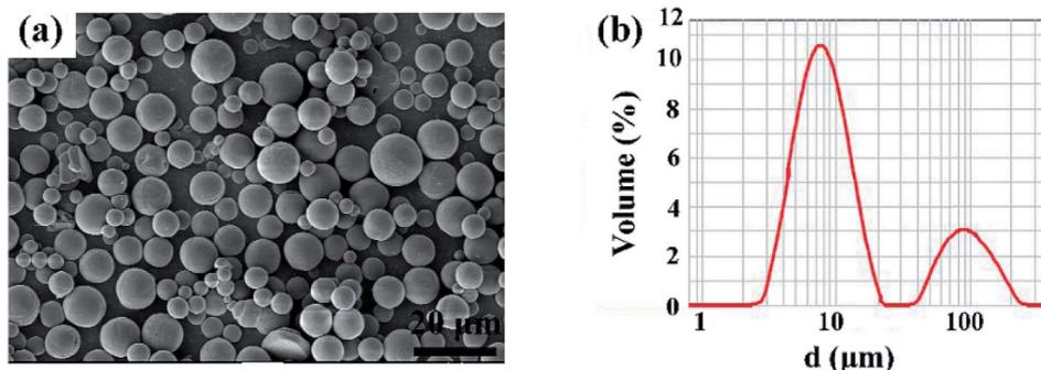
Fig. 3 (a) SEM image; (b) particle size analysis of spherical  $\text{Al}_2\text{O}_3$  powder.
