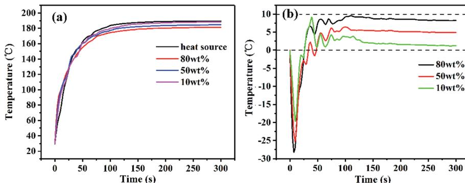
Fig. 7 (a) The center temperature of samples with different filler content at room temperature of  $28^\circ\text{C}$ ; (b) center temperature difference of composites with different filler content.
