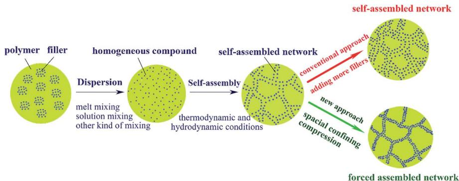
Fig. 1 Scheme of technological pathway of SCFNA method and conventional compounding.<sup>22,23</sup>
