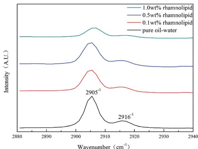
Fig. 10 Raman spectra of hydrate in the presence of rhamnolipid with different concentrations.
