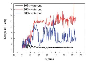
Fig. 5 Torque profiles for different water cuts in pure oil–water system at 275.15 K.
