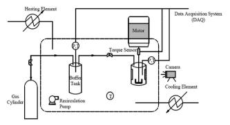
Fig. 2 Schematic diagram of high-pressure visual autoclave apparatus.
