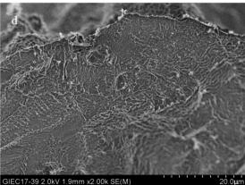
Fig. 11 Microstructure images of hydrate in the presence of rhamnolipid with different concentrations: (a) pure oil–water, (b) 0.1 wt% rhamnolipid, (c) 0.5 wt% rhamnolipid, (d) 1.0 wt% rhamnolipid.
