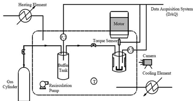
Fig. 2 Schematic diagram of high-pressure visual autoclave apparatus.
