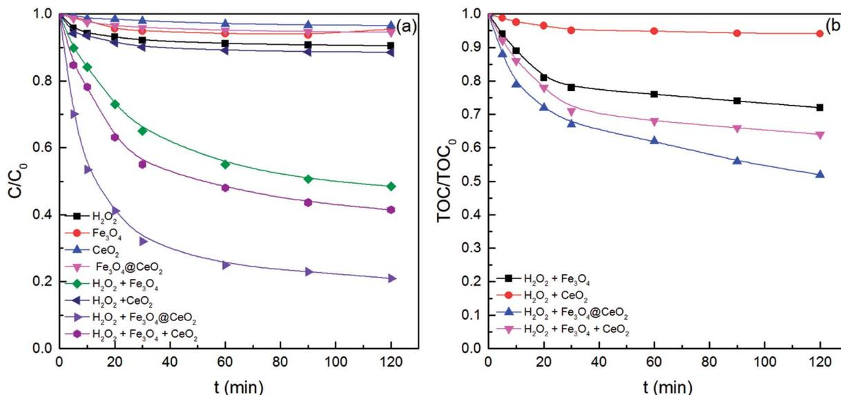
Fig. 4 Removal efficiency of (a) benzoic acid and (b) TOC in different processes. Experimental conditions: 50 mg L<sup>-1</sup> of benzoic acid, 1 g L<sup>-1</sup> of catalyst, 250 mg L<sup>-1</sup> of H<sub>2</sub>O<sub>2</sub>, T = 30 °C, pH = 3.2.
