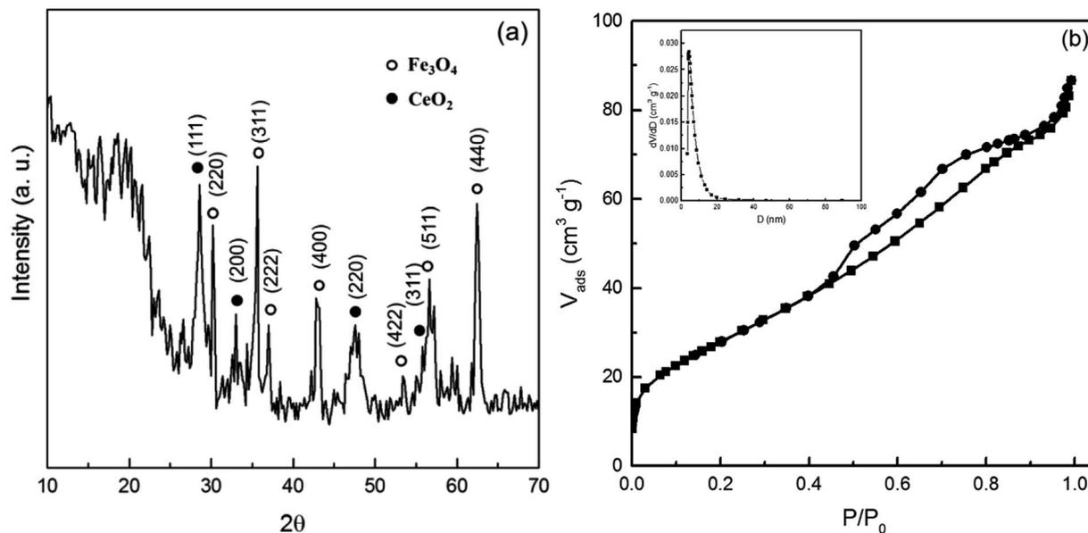
Fig. 1 (a) X-ray pattern of  $\text{Fe}_3\text{O}_4@ \text{CeO}_2$  nanoparticles; (b)  $\text{N}_2$  adsorption–desorption isotherms and pore size distribution (inset) of  $\text{Fe}_3\text{O}_4@ \text{CeO}_2$  nanoparticles.
