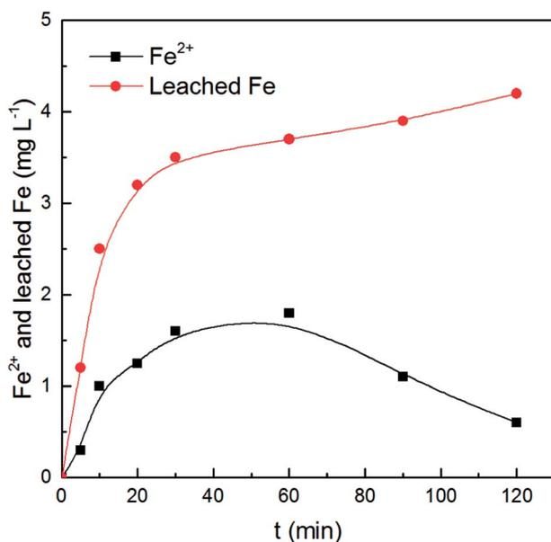
Fig. 6 Variation of the concentration of  $\text{Fe}^{2+}$  and leached Fe in the solution during CWPO of benzoic acid. Experimental conditions:  $50 \text{ mg L}^{-1}$  of benzoic acid,  $1 \text{ g L}^{-1}$  of catalyst,  $250 \text{ mg L}^{-1}$  of  $\text{H}_2\text{O}_2$ ,  $T = 30^\circ\text{C}$ ,  $\text{pH} = 3.2$ .
