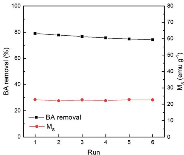
Fig. 8 Benzoic acid removal and the saturation magnetization of  $\text{Fe}_3\text{O}_4@\text{CeO}_2$  catalyst in the stability tests. Experimental conditions:  $50 \text{ mg L}^{-1}$  of benzoic acid,  $1 \text{ g L}^{-1}$  of catalyst,  $250 \text{ mg L}^{-1}$  of  $\text{H}_2\text{O}_2$ ,  $T = 30^\circ\text{C}$ ,  $\text{pH} = 3.2$ .
