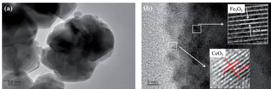
Fig. 2 TEM and HR-TEM images of  $\text{Fe}_3\text{O}_4@\text{CeO}_2$ .
