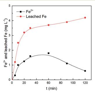
Fig. 6 Variation of the concentration of Fe<sup>2+</sup> and leached Fe in the solution during CWPO of benzoic acid. Experimental conditions:  $50 \text{ mg L}^{-1}$  of benzoic acid,  $1 \text{ g L}^{-1}$  of catalyst,  $250 \text{ mg L}^{-1}$  of  $H_2O_2$ ,  $T = 30 \, ^{\circ}\text{C}$ , PH = 3.2.
