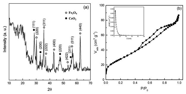
Fig. 1 (a) X-ray pattern of Fe $_3$ O $_4$ @CeO $_2$  nanoparticles; (b) N $_2$  adsorption—desorption isotherms and pore size distribution (inset) of Fe $_3$ O $_4$ @CeO $_2$  nanoparticles.
