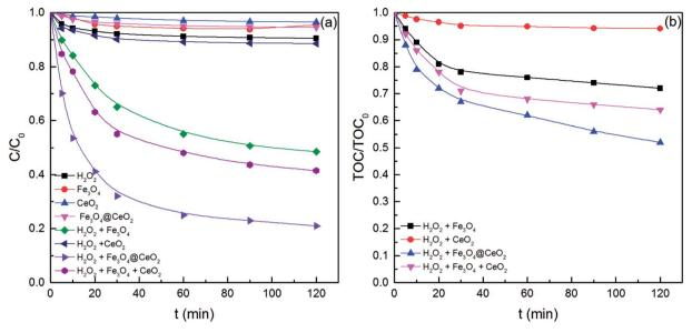
Fig. 4 Removal efficiency of (a) benzoic acid and (b) TOC in different processes. Experimental conditions: 50 mg L $^{-1}$  of benzoic acid, 1 g L $^{-1}$  of catalyst, 250 mg L $^{-1}$  of H $_2$ O $_2$ , T = 30 °C, pH = 3.2.
