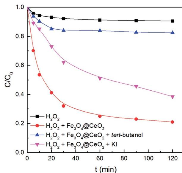
Fig. 7 Effect of radical scavengers on CWPO of benzoic acid. Experimental conditions:  $50 \text{ mg L}^{-1}$  of benzoic acid,  $1 \text{ g L}^{-1}$  of catalyst,  $250 \text{ mg L}^{-1}$  of  $\text{H}_2\text{O}_2$ ,  $T = 30^\circ\text{C}$ ,  $\text{pH} = 3.2$ .
