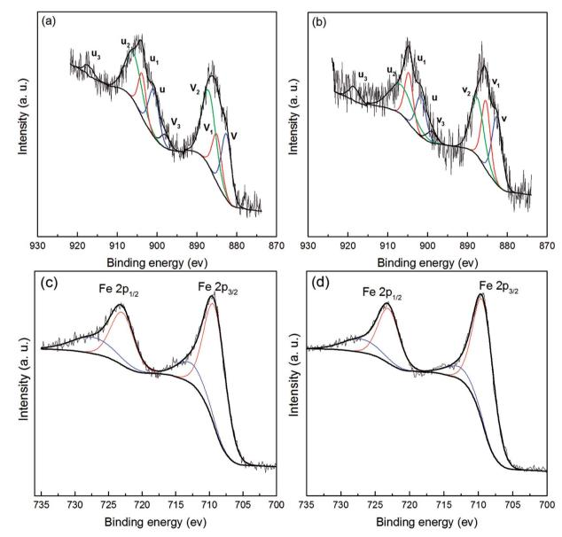
Fig. 3 (a) Ce 3d and (c) Fe 2d XPS spectra of Fe<sub>3</sub>O<sub>4</sub>@CeO<sub>2</sub> before reaction; (b) Ce 3d and (d) Fe 2d XPS spectra of Fe<sub>3</sub>O<sub>4</sub>@CeO<sub>2</sub> after reaction.
