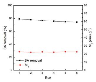
Fig. 8 Benzoic acid removal and the saturation magnetization of  $Fe_3O_4$ @CeO<sub>2</sub> catalyst in the stability tests. Experimental conditions: 50 mg L<sup>-1</sup> of benzoic acid, 1 g L<sup>-1</sup> of catalyst, 250 mg L<sup>-1</sup> of H<sub>2</sub>O<sub>2</sub>, T = 30 °C, pH = 3.2.
