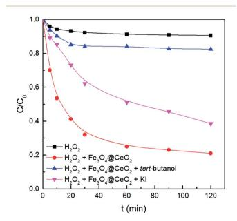
Fig. 7 Effect of radical scavengers on CWPO of benzoic acid. Experimental conditions: 50 mg  $L^{-1}$  of benzoic acid, 1 g  $L^{-1}$  of catalyst, 250 mg  $L^{-1}$  of H<sub>2</sub>O<sub>2</sub>,  $T=30\,^{\circ}\text{C}$ , pH = 3.2.
