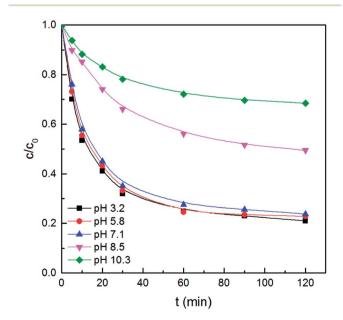
Fig. 5 Effect of solution pH on the degradation of benzoic acid in CWPO with Fe<sub>3</sub>O<sub>4</sub>@CeO<sub>2</sub> catalyst. Experimental conditions: 50 mg L<sup>-1</sup> of benzoic acid, 1 g L<sup>-1</sup> of catalyst, 250 mg L<sup>-1</sup> of H<sub>2</sub>O<sub>2</sub>, T = 30 °C.
