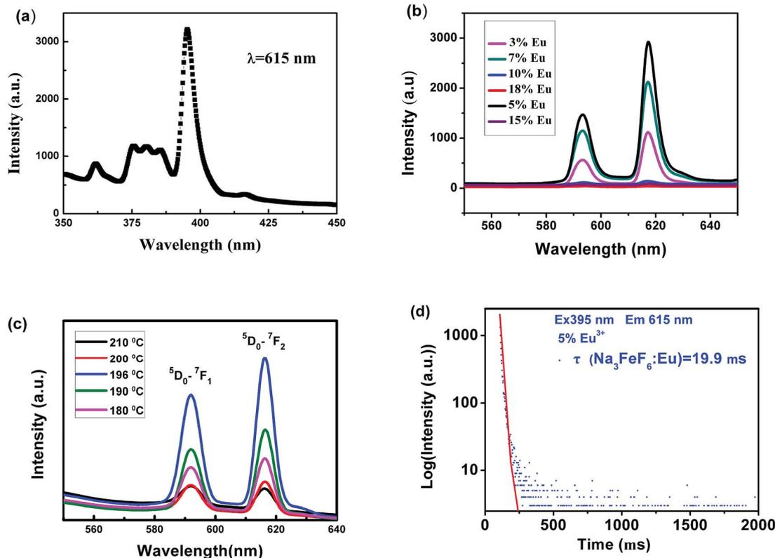
Fig. 6 (a) Excitation spectrum of  $\text{Na}_3\text{FeF}_6$ :5%  $\text{Eu}^{3+}$ . (b) Emission spectra of  $\text{Na}_3\text{FeF}_6$  doped with different concentration of  $\text{Eu}^{3+}$ . (c) Emission spectra of the  $\text{Na}_3\text{FeF}_6$ :5%  $\text{Eu}^{3+}$  synthesized at different temperature. (d) Decay curves of the red (615 nm) emission under pulsed 395 nm excitation for the powder of  $\text{Na}_3\text{FeF}_6$ :5%  $\text{Eu}^{3+}$ .
