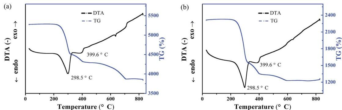
Fig. 3 TG and DTA curves: (a)  $\text{Na}_3\text{FeF}_6$  and (b)  $\text{Na}_3\text{FeF}_6:5\% \text{Eu}^{3+}$ .
