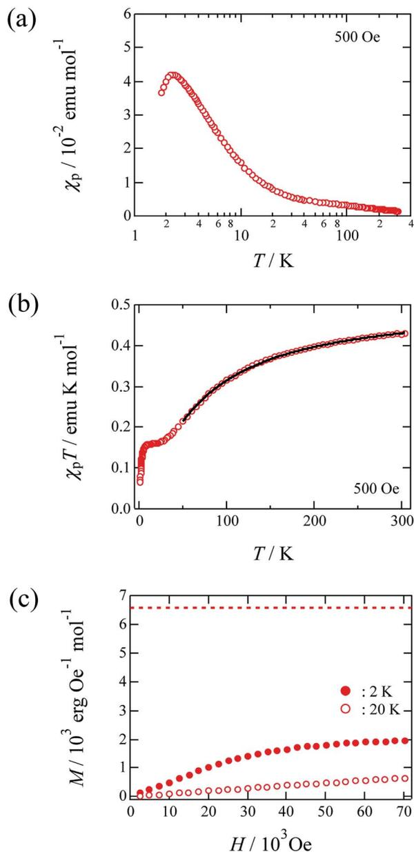
Fig. 3 Magnetic properties of **1**. The molar unit of  $\chi_p$  and magnetization was chosen as the quantity per one mole of Cu. (a) Temperature dependence of the paramagnetic susceptibility  $\chi_p$  for non-oriented microcrystals under 500 Oe. (b) The  $\chi_p T$  vs.  $T$  plot for non-oriented microcrystals. The solid curves indicate the theoretical best fits of eqn (1). (c) Field dependence of the magnetization for non-oriented microcrystals of **1** at 2 K and 20 K.
