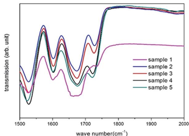
Fig. 1 Transmission FT-IR spectra indicating the presence of thiourethane and urethane in all synthesized nanocarriers (sample 1–5).
