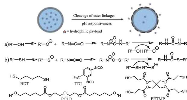
**Scheme 1** A schematic representation of the reaction mechanism between (a) hydroxyl and isocyanate groups, and (b) thiol and isocyanate groups. Both reactions are executed in the presence of a base catalyst.  $R' = PCLD$ ;  $R'' = BDT$  or  $PETMP$ .
