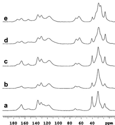
Fig. 2 High-resolution solid-state  $^{13}\text{C}$  NMR data demonstrating the presence of thiourethane for sample 1 (a) and both thiourethane and urethane for samples 2 (b), 3 (c), 4 (d) and 5 (e) (see Table 1).
