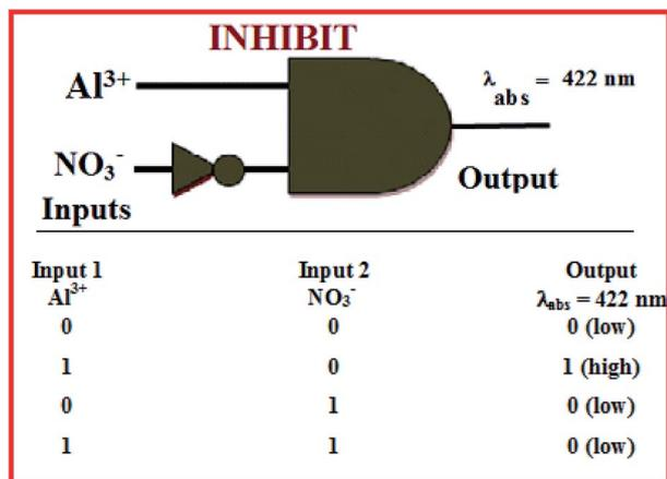
Fig. 13 Logic scheme and the truth table for the proposed INHIBIT type logic gate.
