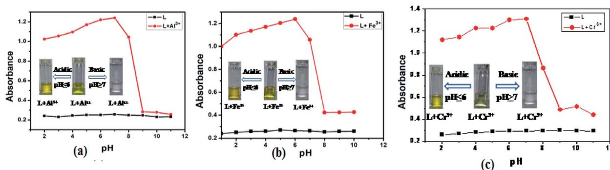
Fig. 10 Absorbance of (a) L, L–Al<sup>3+</sup>, (b) L, L–Fe<sup>3+</sup> and (c) L, L–Cr<sup>3+</sup> at various ranges of pH in CH<sub>3</sub>CN–H<sub>2</sub>O (1 : 1, v/v) at room temperature. Inset: intensity at 422 nm, 422 nm and 416 nm respectively for L–M<sup>3+</sup> (M = Al, Fe and Cr).
