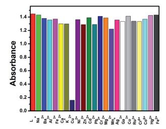
Fig. 9 Competitive selectivity of  $L^{\prime}$  towards  $Cu^{2+}$  in the presence of other metal ions.
