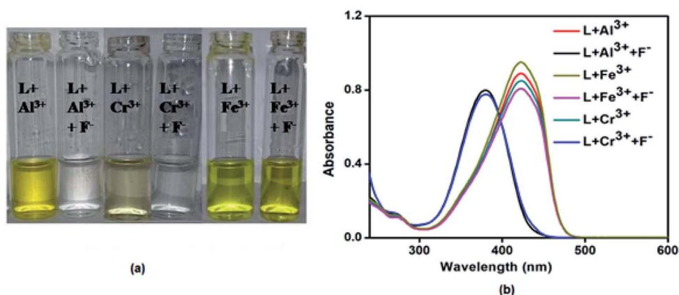
Fig. 12 Reversibility study of L towards Al<sup>3+</sup>, Fe<sup>3+</sup> and Cr<sup>3+</sup> ions using 5 equiv. of KF (a) through color change (b) absorbance change.
