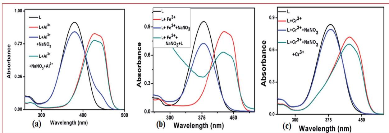
Fig. 11 Absorbance spectra of L in the absence and presence of (a) Al<sup>3+</sup>/NaNO<sub>3</sub>, (b) Fe<sup>3+</sup>/NaNO<sub>3</sub> and (c) Cr<sup>3+</sup>/NaNO<sub>3</sub>, respectively in CH<sub>3</sub>CN–H<sub>2</sub>O (1 : 1, v/v).
