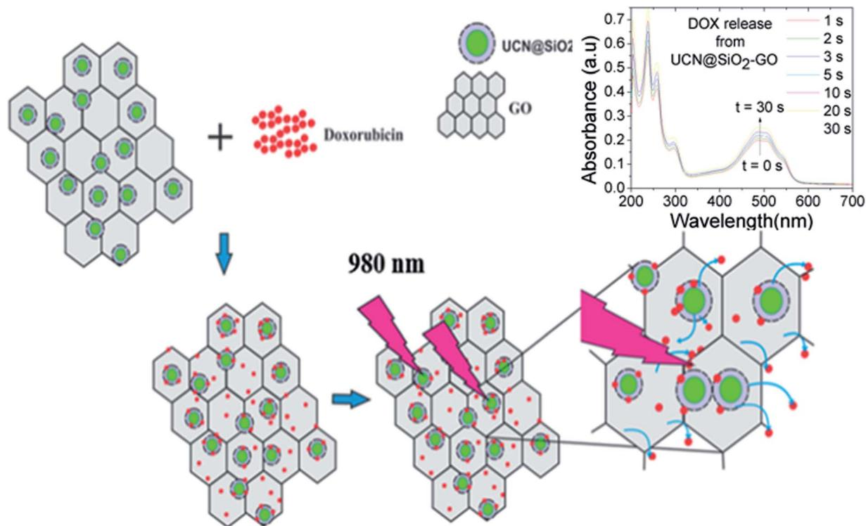
**Scheme 2** Represents the procedure and mechanism of control release of DOX from UCN@SiO<sub>2</sub>-GO. Release of DOX has been controlled by 980 nm NIR laser pulse.
