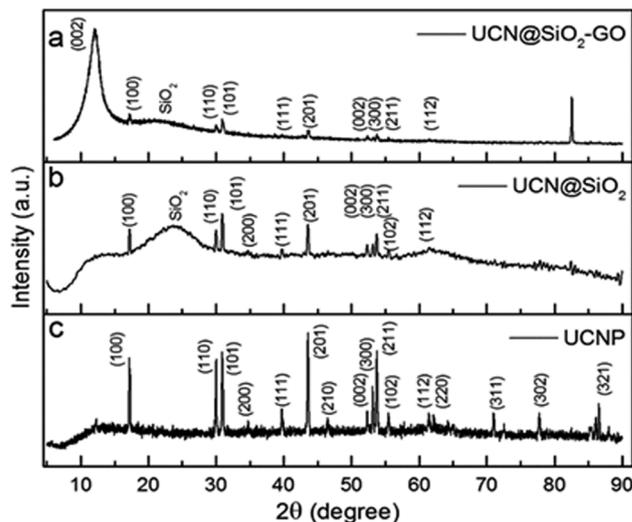
Fig. 5 XRD spectra of UCNPs, UCN@SiO<sub>2</sub> NPs and UCN@SiO<sub>2</sub>-GO nanocomposite.
