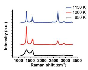
Fig. 3 Raman spectra of the grown films after the transfer onto  $SiO_2/Si$  substrate. All spectra were normalized to the intensity of G band.
