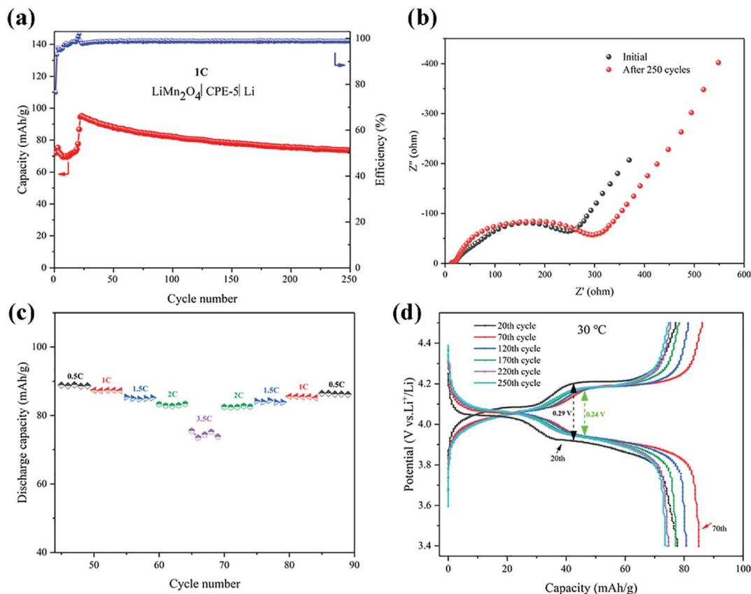
Fig. 6 (a) Cycling performance of a Li|CPE-5|LiMn<sub>2</sub>O<sub>4</sub> cell at 1C. (b) EIS spectra before and after 250 cycles. (c) Rate performance of a Li|CPE-5|LiMn<sub>2</sub>O<sub>4</sub> cell. (d) Typical charge–discharge curves of a Li|CPE-5|LiMn<sub>2</sub>O<sub>4</sub> cell.
