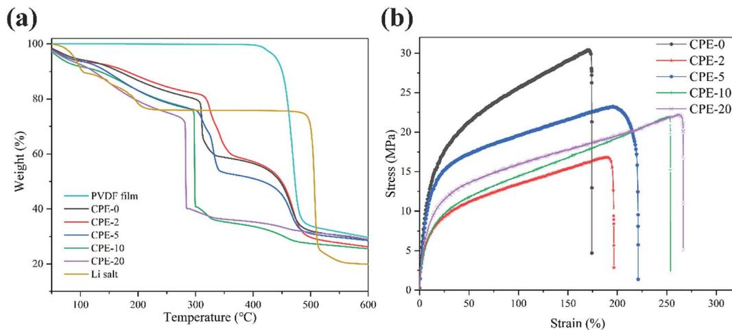
Fig. 3 (a) Thermogravimetric analysis of the pure PVDF film, CPEs and LiClO<sub>4</sub>. (b) Stress–strain curves of CPEs.
