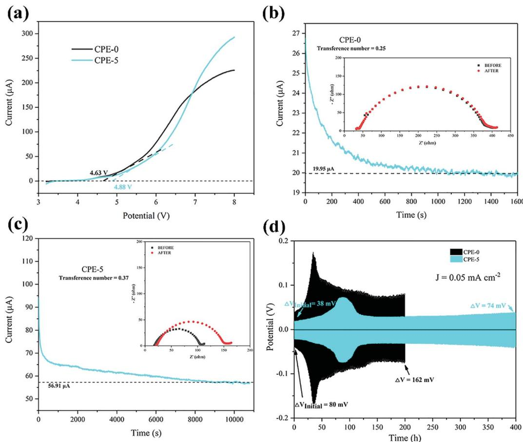
Fig. 5 (a) LSV plots of CPE-0 and CPE-5 at a scanning rate of  $10 \text{ mV s}^{-1}$ . (b and c) Chronoamperometry of the Li|CPEs|Li cells at a potential of 10 mV. EIS spectra of the cells before and after the polarization are shown in the inset. (d) Galvanostatic cycles with a constant current density of  $0.05 \text{ mA cm}^{-2}$  for the Li|CPEs|Li cells.
