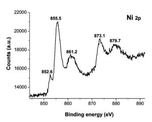
Fig. 1 X-ray photoelectron spectroscopy (XPS) spectra of Ni<sub>2</sub>P.
