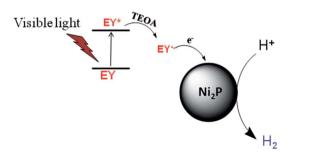
Fig. 5 Schematic illustration of probable mechanism of photosensitized hydrogen production. Noted that EY\*, EY\*-, TEOA represent the triplet excited state of Eosin Y, the radical anion of Eosin Y and triethanolamine, respectively
