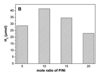
Fig. 6 Effect of (A) initial EY concentration and (B) mole ratio of initial P/Ni on hydrogen evolution of EY sensitized Ni<sub>2</sub>P.
