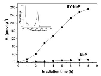
Fig. 4 Time courses of photocatalytic  $H_2$  production of EY- $Ni_2P$  and  $Ni_2P$ . Conditions: 0.10 g  $Ni_2P$ , 9.5  $\times$  10<sup>-2</sup> mol L<sup>-1</sup> TEOA, light source: 150 W high pressure Hg lamp,  $\lambda$  > 420 nm. The inset is UV-Vis absorption spectra of EY.
