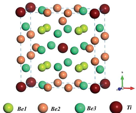
Fig. 1 Schematic of the unit cell of the  $\text{Be}_{12}\text{Ti}$  crystal structure; red balls, yellow balls, orange balls, and green balls denote Be1 atoms, Be2 atoms, Be3 atoms, and Ti atoms, respectively.
