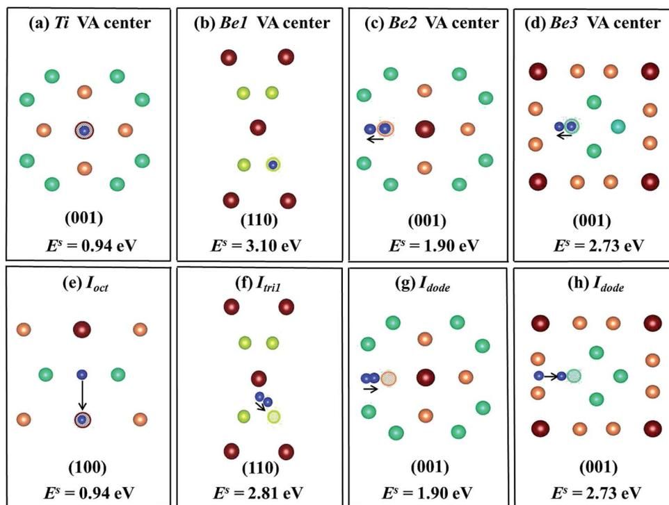
Fig. 6 Schematic diagrams and corresponding solution energies of a single He atom in the vacancy centers ((a)–(d)) and interstitial sites near vacancies ((e)–(h)) in the Be<sub>12</sub>Ti solid. The hollow circles of different colours represent corresponding vacancies and dark blue balls denote He atoms.
