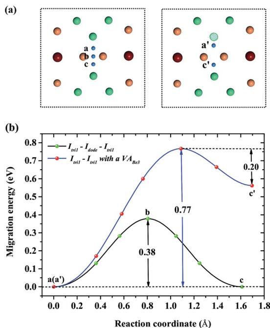
Fig. 9 (a) Diffusion paths  $I_{\text{tri1}}-I_{\text{dode}}-I_{\text{tri1}}$  and  $I_{\text{tri1}}-I_{\text{tri1}}$  with a  $V_{\text{Be3}}$  for H atoms. (b) Corresponding migration energy profiles.
