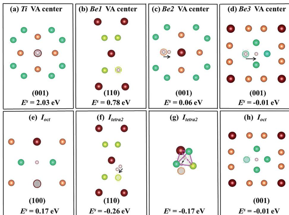
Fig. 4 Schematic diagrams and corresponding solution energies of a single H atom in the vacancy centers ((a)–(d)) and interstitial sites near vacancies ((e)–(h)) in the Be<sub>12</sub>Ti solid. The hollow circles of different colours represent the corresponding vacancies and pink balls denote H atoms.
