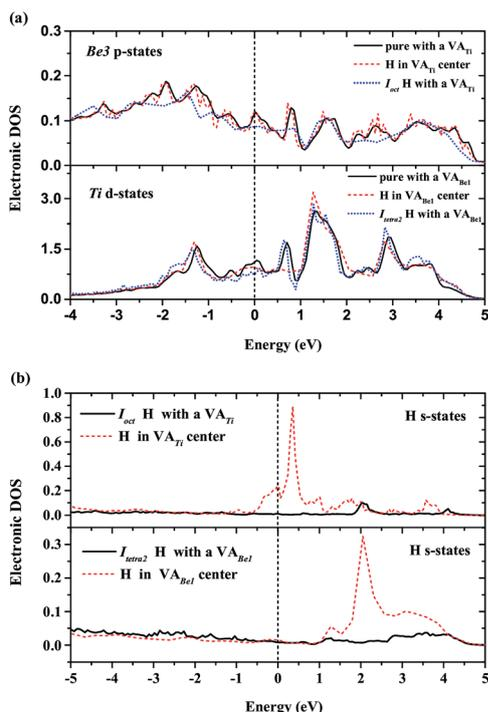
Fig. 5 (a) Local DOS for vacancy nearest-neighbor Ti and Be3 atoms; (b) local DOS for interstitial H atoms within VA<sub>Ti</sub> and VA<sub>Be1</sub>. The Fermi energy of the supercell with the H defect is 0.00 eV.
