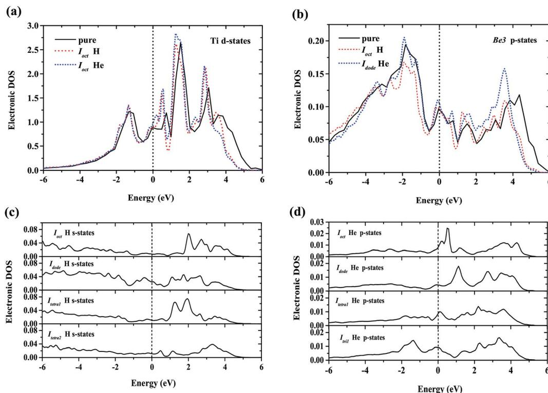
Fig. 3 (a) Local DOS for H/He nearest-neighbor Ti atom; (b) local DOS for H/He nearest-neighbor Be3 atom; (c) local DOS for interstitial H atoms – the s-projected DOS of H at  $I_{\text{oct}}$ ,  $I_{\text{dode}}$ ,  $I_{\text{tetra1}}$ , and  $I_{\text{tetra2}}$ ; (d) local DOS for interstitial He atoms – the p-projected DOS of He at  $I_{\text{oct}}$ ,  $I_{\text{dode}}$ ,  $I_{\text{tetra1}}$ , and  $I_{\text{trt1}}$ . The Fermi energy of the supercell with the H/He defect is 0.00 eV.
