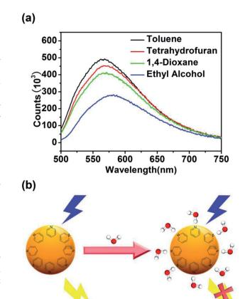
Fig. 6 (a) The fluorescence emission spectra (excited by the light of 440 nm) of CQDs dispersed in different organ solvents (toluene, tetrahydrofuran, 1,4-dioxane, ethanol); (b) schematic illustration for the detection of  $H_2O$  in organic solvents by CQDs.
