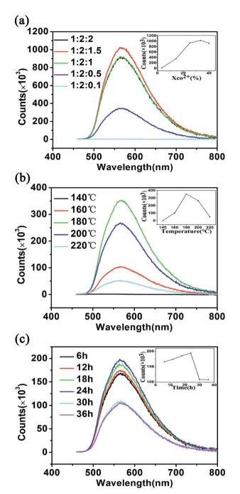
Fig. 1 Effects of (a) mass fraction of cobalt chloride, (b) reaction temperature, and (c) reaction time on the fluorescence intensity.
