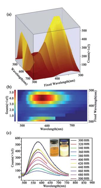
Fig. 4 (a) The fluorescence emission–excitation 3D map of the asprepared CQDs; (b) the contour plot of photoluminescence spectrum for CQDs; (c) photoluminescence spectrum of the as-prepared CQDs (inset: photographs of CQDs toluene solutions exposed to daylight (left) and 365 nm UV radiation (right)).
