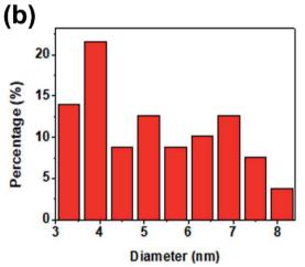
**Fig. 2** (a) The TEM image of CQDs (the inset shows the high resolution TEM images of single CQD), (b) the corresponding particle size distribution histogram of (a).
