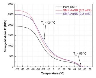
Fig. 2 Tensile storage modulus (E') as a function of temperature for SMP, SMP/AuNS (0.2 wt%), and SMP/AuNR (0.2 wt%) nanocomposites. The glass transitions and the melting transitions were approx. -24 °C and 55 °C, respectively for all the SMP and SMP/AuNP composites.
