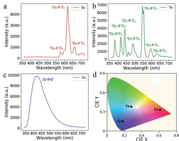
Fig. 6 Emission spectra of the additive manufactured glass doped with (a)  $\text{Eu}^{3+}$ , (b)  $\text{Tb}^{3+}$  and (c)  $\text{Ce}^{3+}$  ions under the excitation at 254 nm. (d) The CIE coordinate of the RE-doped glasses.
