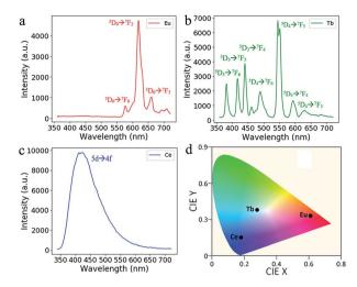
Fig. 6 Emission spectra of the additive manufactured glass doped with (a)  $Eu^{3+}$ , (b)  $Tb^{3+}$  and (c)  $Ce^{3+}$  ions under the excitation at 254 nm. (d) The CIE coordinate of the RE-doped glasses.
