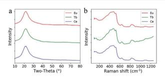
Fig. 4 (a) XRD patterns of the doped silica glass. (b) Raman spectra of the doped silica glass.
