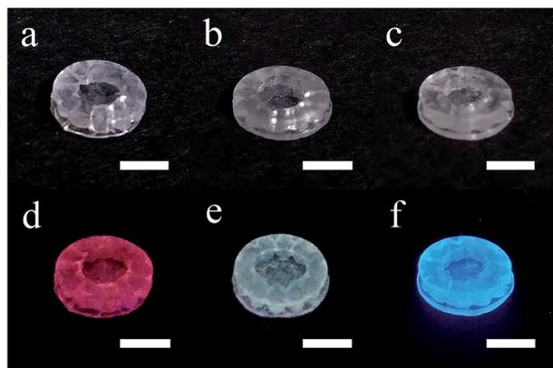
Fig. 5 Photos of the additive manufactured silica glass doped with (a)  $\text{Eu}^{3+}$ , (b)  $\text{Tb}^{3+}$  and (c)  $\text{Ce}^{3+}$  ions and (d–f) their luminescent performance under a 254 nm UV lamp. The scale bars represent 5 mm.
