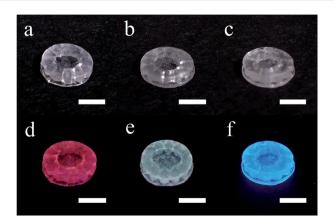
Fig. 5 Photos of the additive manufactured silica glass doped with (a)  $Eu^{3+}$ , (b)  $Tb^{3+}$  and (c)  $Ce^{3+}$  ions and (d-f) their luminescent performance under a 254 nm UV lamp. The scale bars represent 5 mm.
