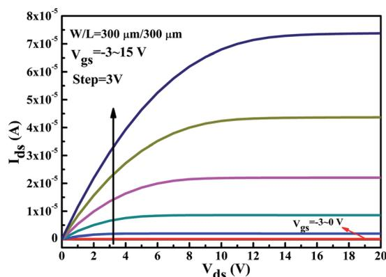
Fig. 8 The Output curves of ITZO TFT annealed at 300 °C in air for 90 min.
