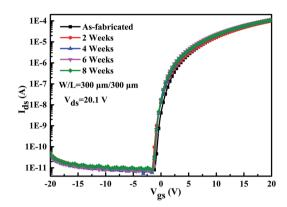
Fig. 9 The evolution of the transfer curves for the ITZO TFTs with annealing temperature of 300 °C without any passivation in air for 8 weeks.
