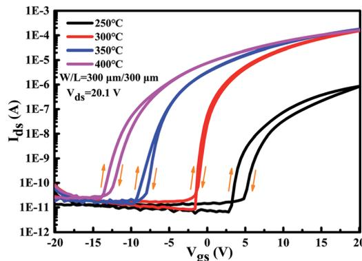
Fig. 7 The transfer characteristics of the fabricated ITZO TFTs with respect to various annealing temperatures (at 250 °C, 300 °C, 350 °C, and 400 °C).
