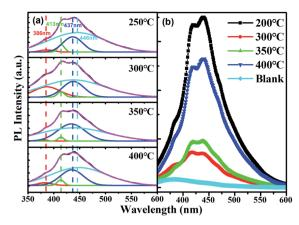
Fig. 5 (a) Gaussian fitting is illustrated using the spectrum of ITZO film treated at different temperatures ( $250 \,^{\circ}$ C,  $300 \,^{\circ}$ C,  $350 \,^{\circ}$ C, and  $400 \,^{\circ}$ C). (b) PL spectra of ITZO films annealed in air for 90 min at different temperatures and a blank glass substrate.
