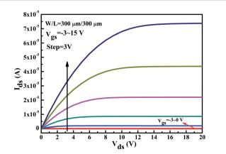
Fig. 8 The Output curves of ITZO TFT annealed at 300 °C in air for 90 min.
