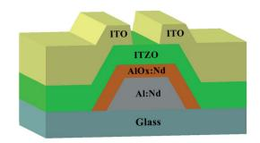
Fig. 1 Schematic diagram of the sputtered ITZO thin film transistor.
