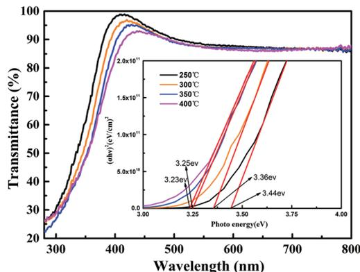
Fig. 4 Optical properties of ITZO films deposited at room temperature onto glass substrates at various annealing temperatures in the range of 250–400 °C. Inset: the plot of  $(\alpha hv)^2$  as a function of  $hv$ .
