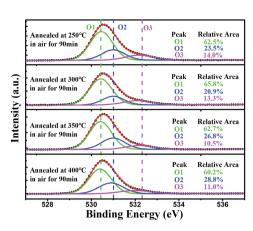
Fig. 6 XPS O 1s spectra with fitted curves (O1, O2, and O3 sub-peaks) and the relatively area ratio of O1, O2, and O3 peaks obtained from the ITZO thin-films annealed at various temperatures (250  $^{\circ}$ C, 300  $^{\circ}$ C, 350  $^{\circ}$ C, and 400  $^{\circ}$ C).
