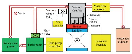
Fig. 4 Simplified schematic diagram of the FCD instrument.
