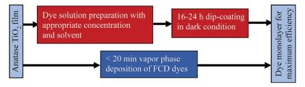
Fig. 1 Comparison of FCD<sup>6</sup> and conventional dip-coating dye loading processes
