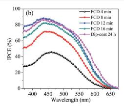
Fig. 6 Comparison of incident photon-to-current conversion efficiency (IPCE) for dip-coating and FCD-based DSSCs (a) IPCE spectra of L1 dye based DSSCs; peak IPCE increased with increased FCD duration until reached an optimum duration of 16 min (b) IPCE spectra of L2 dye based DSSCs; peak IPCE increased with increased FCD duration until reached an optimum duration of 12 min.
