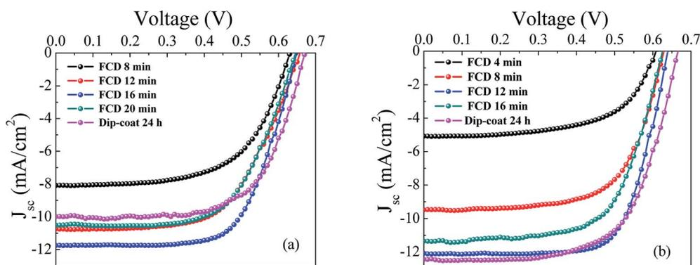
Fig. 5 Comparison of photovoltaic performance for dip-coating and FCD-based DSSCs (a) *J*–*V* curves of L1-based DSSCs; an optimum 16 min FCD shows significantly better performance compared to 24 h dip-coating (b) *J*–*V* curves of L2-based DSSCs; an optimum 12 min FCD shows equivalent performance to 24 h dip-coating.
