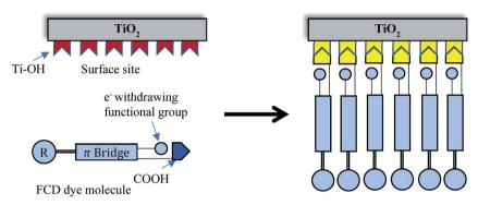
Fig. 2 An FCD dye molecule attaches through a -COOH group with surface -OH site
