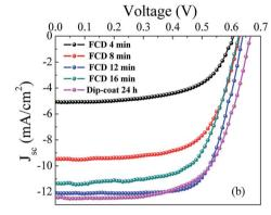
Fig. 5 Comparison of photovoltaic performance for dip-coating and FCD-based DSSCs (a) J-V curves of L1-based DSSCs; an optimum 16 min FCD shows significantly better performance compared to 24 h dip-coating (b) J-V curves of L2-based DSSCs; an optimum 12 min FCD shows equivalent performance to 24 h dip-coating.
