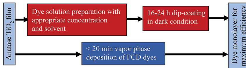
Fig. 1 Comparison of FCD<sup>6</sup> and conventional dip-coating dye loading processes.
