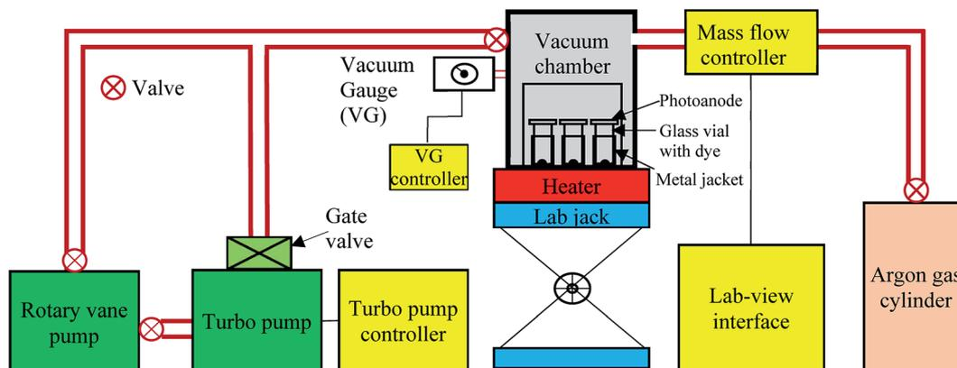
Fig. 4 Simplified schematic diagram of the FCD instrument.
