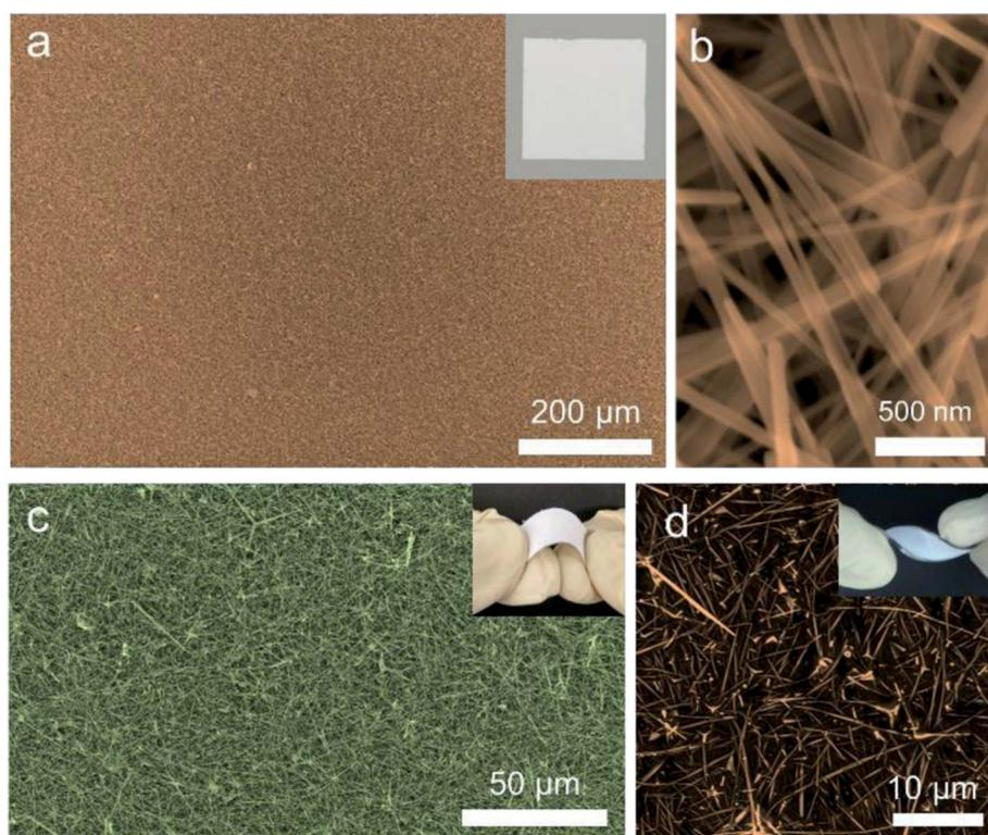
**Fig. 2** ZnO NW networks on various substrates. (a) Large-area SEM images of the ZnO NW network film transferred on a glass substrates, inset: photograph of ZnO NW network film on a glass substrate. (b) High magnification SEM image of ZnO NWs on a glass substrate. SEM images of the ZnO NW network film transferred onto (c) PET and (d) PDMS substrates, insets: the corresponding photograph of ZnO NW network film on PET and PDMS substrates, respectively.
