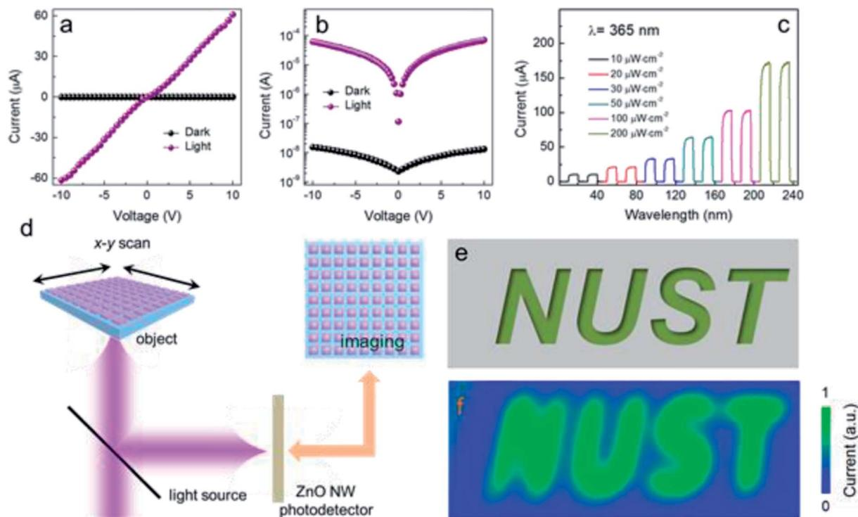
Fig. 3 Imageable photoelectric response characteristics of ZnO NW network. (a)  $I$ - $V$  and (b)  $I$ - $V$  logarithm characteristics of ZnO NW PD in the dark and under 365 nm ( $0.35 \text{ mW cm}^{-2}$ ) illumination. (c)  $I$ - $t$  curves at 5 V of ZnO NW PD under 365 nm with different light irradiation intensity. (d) Schematic of the PD imaging setup. (e) Object and (f) image acquired from the ZnO nanowire PD at  $\lambda$  of 365 nm.
