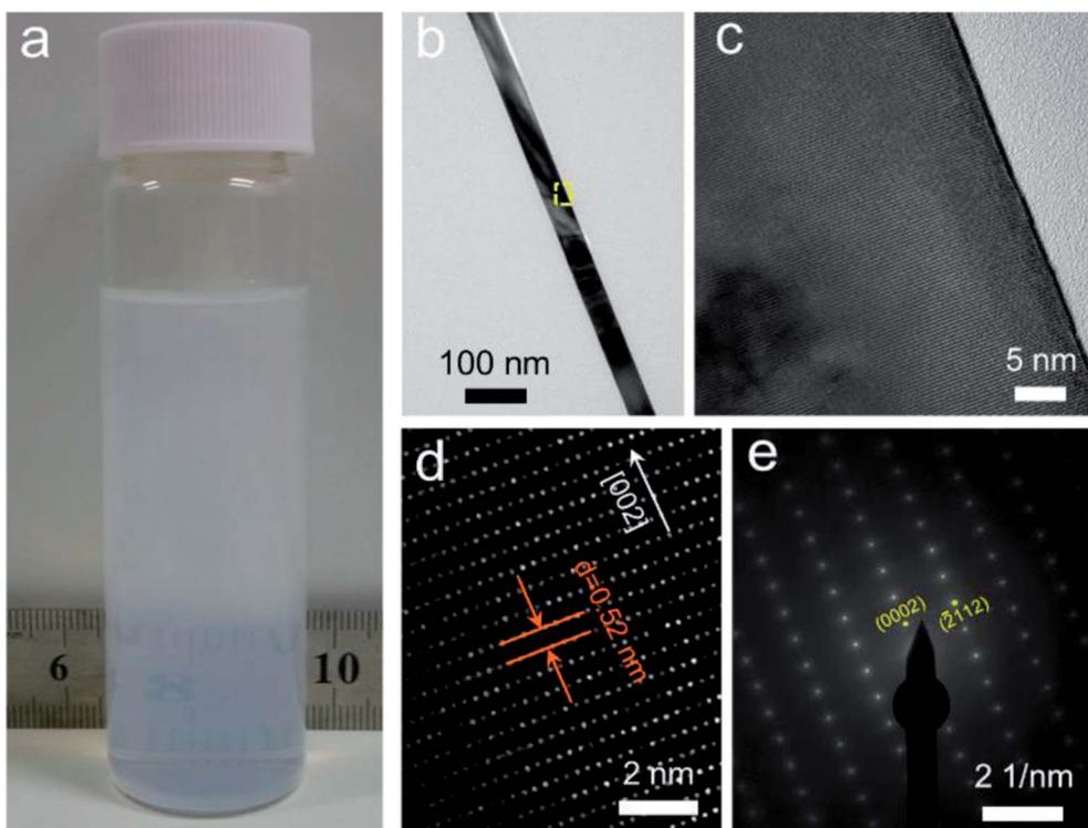
**Fig. 1** (a) Photograph of ZnO NW inks re-dispersed in isopropanol. (b) TEM image of a ZnO NW with diameter of about 35 nm. (c) Magnified TEM image of the surface of a ZnO NW. (d) High-resolution TEM image and (e) SAED pattern of ZnO NWs.
