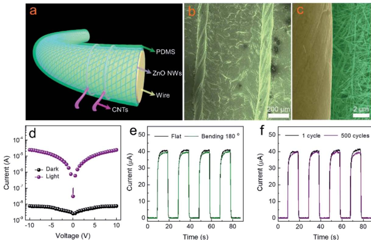
Fig. 6 (a) Device structure of wire-shaped ZnO PD. (b) SEM image and (c) high magnification SEM image of wire-shaped ZnO PD. (d)  $I$ - $V$  logarithm characteristics of ZnO wire-shaped NW PD in the dark and under 365 nm ( $0.35 \text{ mW cm}^{-2}$ ) illumination. (e)  $I$ - $t$  curves at 2 V of ZnO NW PD under 365 nm after bending and recovering cycles. (f)  $I$ - $t$  curves at 2 V of ZnO NW PD under 365 nm with different cycle times.
