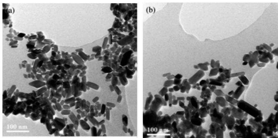
Fig. 7 TEM images of  $\text{TiO}_2$  nanoparticles after hydrothermal treatment of TBA peptized gel at (a) 210 °C and (b) 270 °C.<sup>133</sup>
