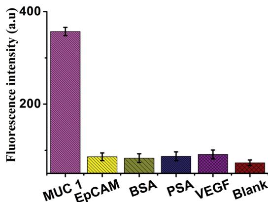
Fig. 6 Fluorescence intensity (at the emission wavelength of 519 nm) of the sensor in the presence of MUC1 (5  $\text{ng mL}^{-1}$ ), EpCAM (50  $\text{ng mL}^{-1}$ ), BSA (50  $\text{ng mL}^{-1}$ ), PSA (50  $\text{ng mL}^{-1}$ ), VEGF (50  $\text{ng mL}^{-1}$ ) and black, respectively. Error bars: SD,  $n = 3$ .
