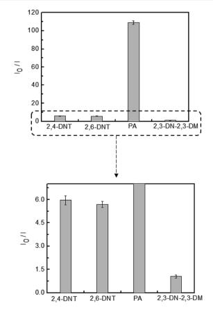
Fig. 5 Relative changes in fluorescence intensity of TPE-CMP (0.375 mg mL $^{-1}$  in CH $_2$ Cl $_2$ ) upon exposure to 2,4-DNT, 2,6-DNT, PA, and 2,3-DN-2,3-DM. [Explosives] = 2.5  $\times$  10 $^{-3}$  M. Excitation wavelength 330 nm.  $I_0$  and I represent fluorescence intensity at 550 nm before and after exposure to explosives, respectively.
