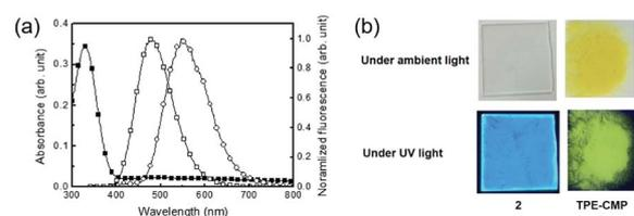
Fig. 3 (a) Absorption (■) and fluorescence spectra (□) of solid **2** and fluorescence spectrum (○) of TPE-CMP, excitation wavelength 330 nm. (b) Photographs of **2** and TPE-CMP under ambient and UV lights (365 nm).
