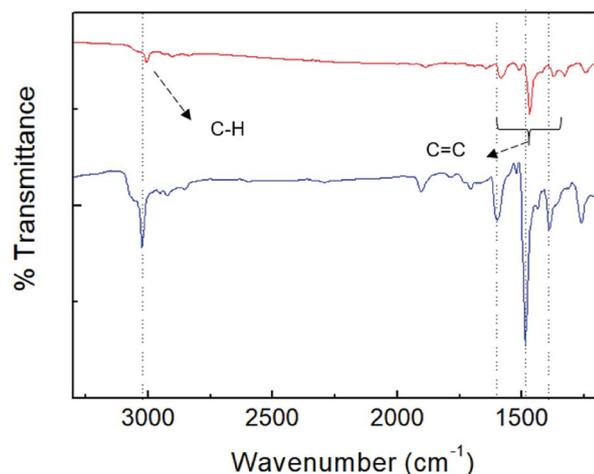
Fig. 7 FT-IR spectra of TPE-CMP before (blue) and after (red) exposure to PA.
