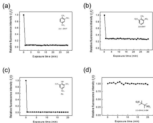
Fig. 4 Changes in the relative fluorescence intensities ( $I_x/I_0$ ) of 1 : 2 TPE-CMP ( $0.375 \text{ mg mL}^{-1}$  in  $\text{CH}_2\text{Cl}_2$ ) upon various exposure time in the presence of (a) 2,4-DNT, (b) 2,6-DNT, (c) PA, and (d) 2,3-DN-2,3-DM. [Explosives] =  $2.5 \times 10^{-3} \text{ M}$ . Excitation wavelength 330 nm.  $I_0$  and  $I_x$  represent fluorescence intensity at 550 nm in the absence and presence of explosives, respectively.
