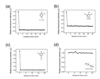
Fig. 4 Changes in the relative fluorescence intensities  $(I_x/I_i)$  of 1:2 TPE-CMP (0.375 mg mL<sup>-1</sup> in CH<sub>2</sub>Cl<sub>2</sub>) upon various exposure time in the presence of (a) 2,4-DNT, (b) 2,6-DNT, (c) PA, and (d) 2,3-DN-2,3-DM. [Explosives] =  $2.5 \times 10^{-3}$  M. Excitation wavelength 330 nm.  $I_i$  and  $I_x$  represent fluorescence intensity at 550 nm in the absence and presence of explosives, respectively.
