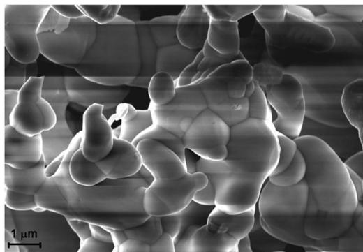
**Fig. 2** A typical FE-SEM image of LLS:0.3%Mn<sup>4+</sup> phosphors.
