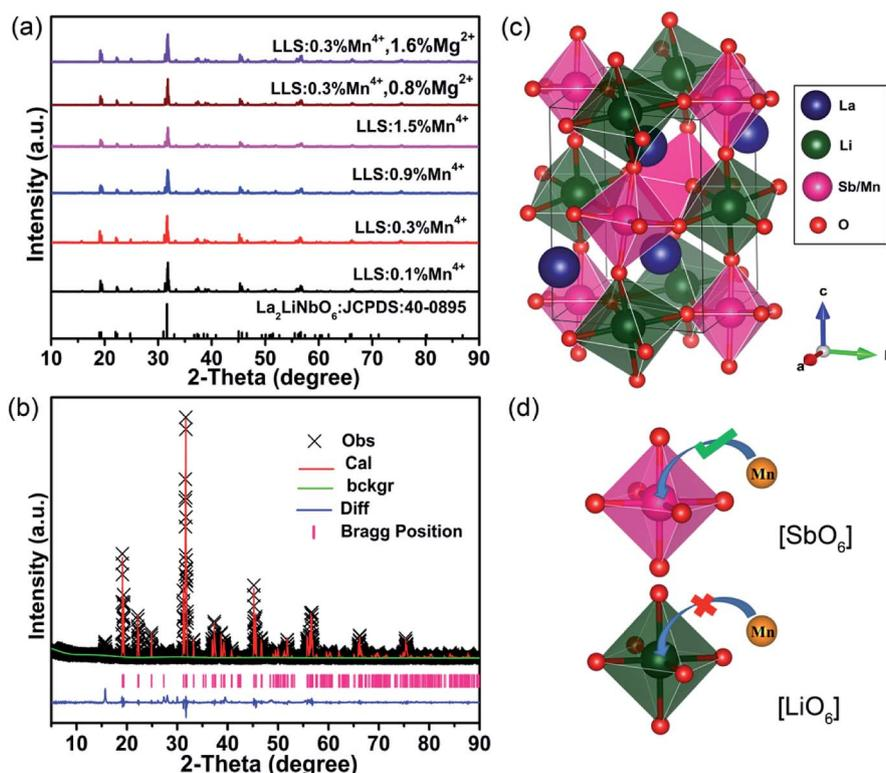
Fig. 1 (a) XRD patterns of the LLS: $x\text{Mn}^{4+}$ ,  $y\text{Mg}^{2+}$  phosphors. (b) Rietveld refinement XRD pattern of the LLS:0.3% $\text{Mn}^{4+}$  phosphors. (c) The structure of the LLS:0.3% $\text{Mn}^{4+}$  phosphors. (d) The octahedron configuration diagrams of  $[\text{SbO}_6]$  and  $[\text{LiO}_6]$ .
