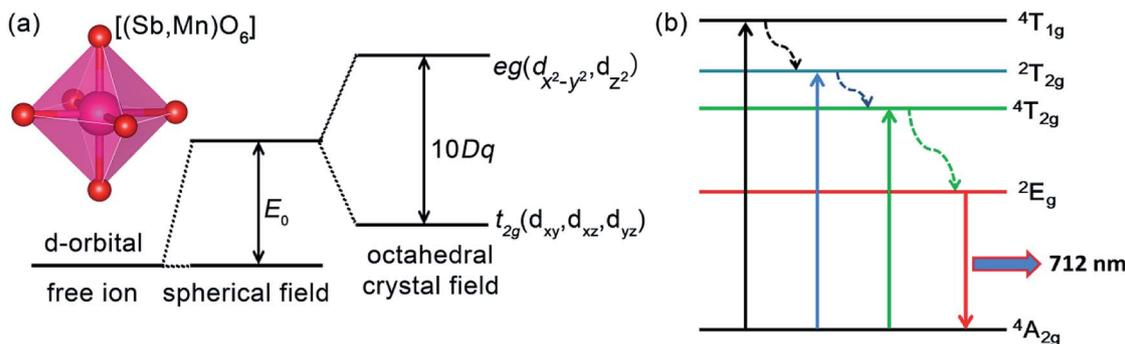
Fig. 6 (a) The simple schematic diagram of the d-orbital splitting in octahedral crystal field with octahedral structure of  $[(\text{Sb},\text{Mn})\text{O}_6]$ . (b) A simple schematic diagram of  $\text{Mn}^{4+}$  ions energy level.
