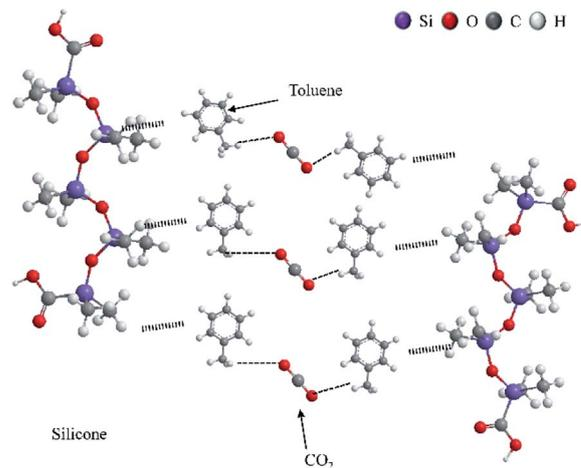
Fig. 12 Thickening mechanism of silicone polymer in liquid CO<sub>2</sub>.
