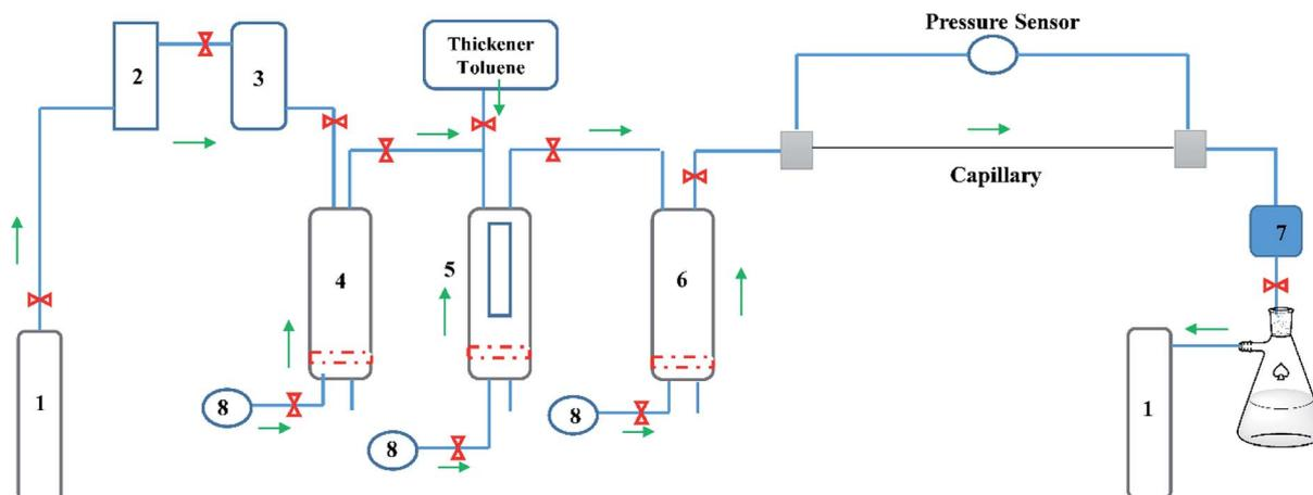
Fig. 4 Capillary viscometers (schematic). (1)  $\text{CO}_2$  cylinder. (2) Desiccator. (3) Compression pump. (4) Pressure-resistant gas cylinder. (5) Dissolution-measuring device. (6) Fracturing fluid-storage device. (7) Pressure-control device. (8) ISCO pump.
