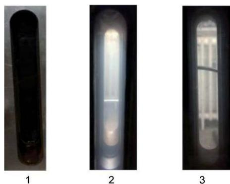
Fig. 10 Phase behavior of liquid CO<sub>2</sub> containing the siloxane and 3-fold toluene (wt%). (1) Deep turbid state. (2) Mild turbid state. (3) Clarified state.
