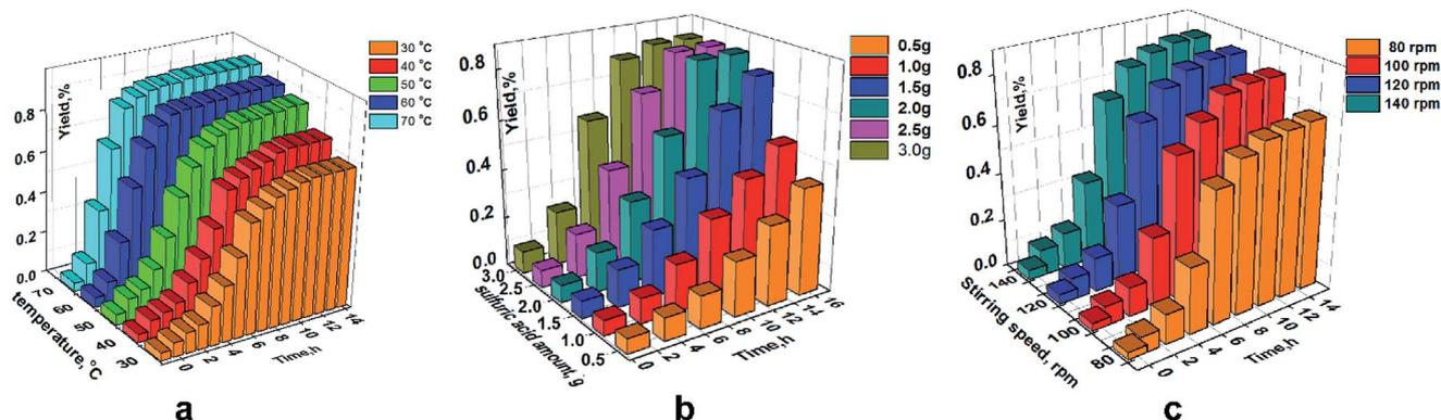
Fig. 6 The effect factors have individually on the yield (ring-opening polymerization). (a) Amount of sulfuric acid is 2.0 g and a stirring speed is 120 rpm. (b) At a temperature of  $70^\circ C$  and a stirring speed of 120 rpm. (c) At a temperature of  $70^\circ C$  and sulfuric acid of 2.0 g.
