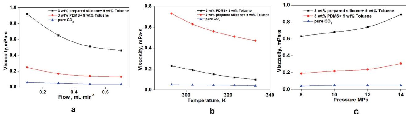
Fig. 11 Effect of different factors on the viscosity of thickened CO<sub>2</sub>. (a) Effect of flow rate at 8 MPa and 303 K; (b) temperature effect at 8 MPa and 0.3 mL min<sup>-1</sup>; (c) pressure effect at 303 K and 0.3 mL min<sup>-1</sup>.
