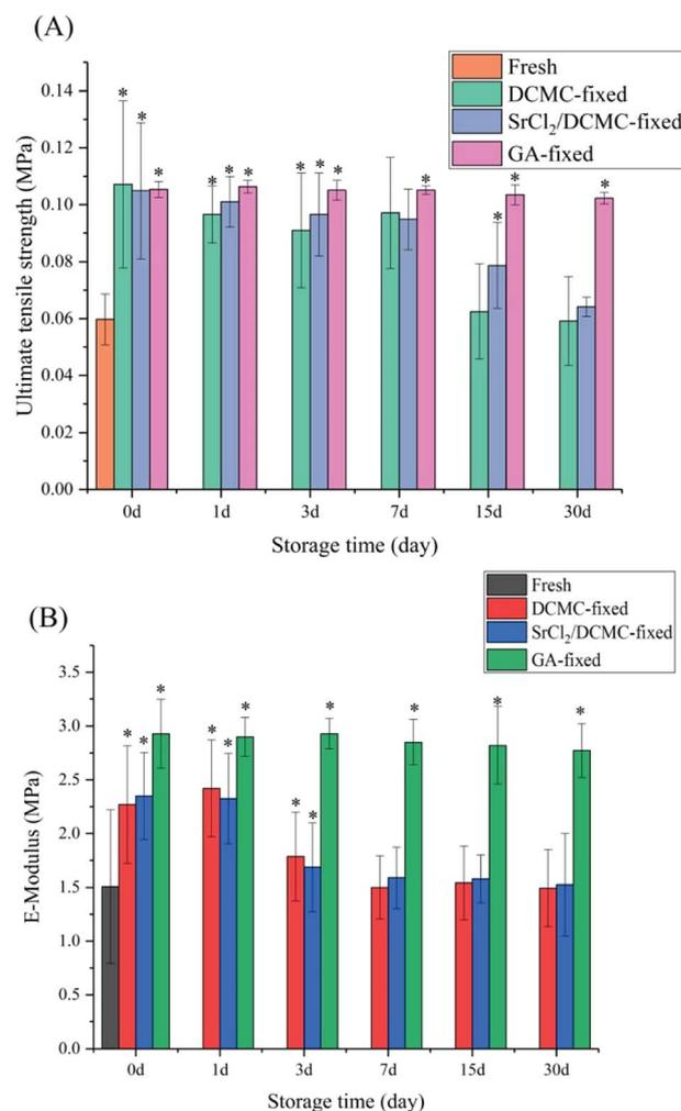
Fig. 3 (A) Ultimate tensile strength and (B) E-modulus of fresh, DCMC-fixed, SrCl<sub>2</sub>/DCMC-fixed and GA-fixed arteries soaking in D-Hanks solution for different period (0 d, 1 d, 3 d, 7 d, 15 d and 30 d, respectively).
