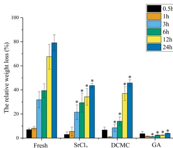
Fig. 6 The relative weight loss of fresh, DCMC-fixed, SrCl<sub>2</sub>/DCMC-fixed and GA-fixed tissues *in vitro* at different time points.
