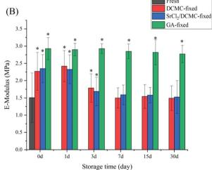
Fig. 3 (A) Ultimate tensile strength and (B) E-modulus of fresh, DCMC-fixed,  $SrCl_2/DCMC$ -fixed and GA-fixed arteries soaking in D-Hanks solution for different period (0 d, 1 d, 3 d, 7 d, 15 d and 30 d, respectively).
