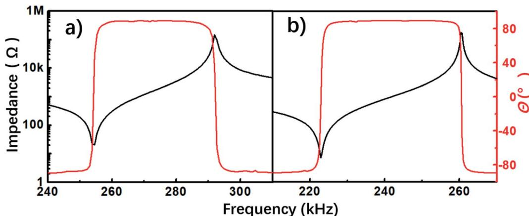
Fig. 3 Impedance  $|Z|$  and phase angle  $\theta$  spectra of PZT-PMnN ceramics prepared by different sintering methods measured as a function of the frequency of PZT-PMnN ceramics prepared by different sintering methods.
