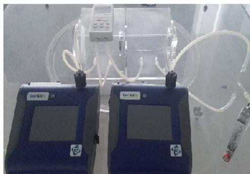
Fig. 2 Schematic diagram and photo-image of the experimental setup for PM<sub>2.5</sub> removal experiment.
