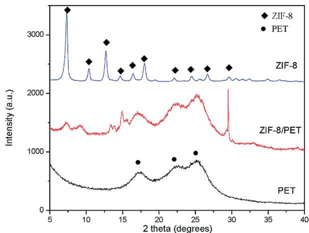
Fig. 3 XRD patterns of ZIF-8, PET and ZIF-8/PET.
