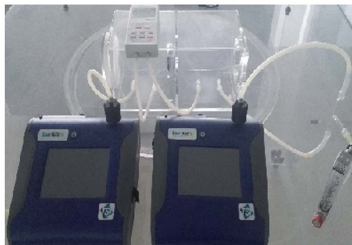
Fig. 2 Schematic diagram and photo-image of the experimental setup for PM 2.5 removal experiment.
