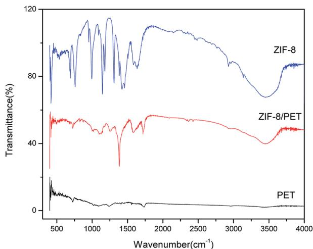
Fig. 6 FT-IR spectra of ZIF-8, PET and ZIF-8/PET.
