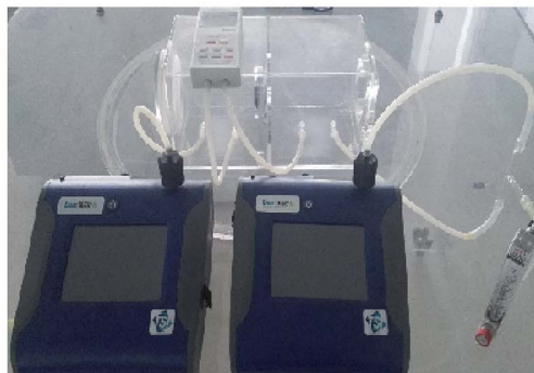
Fig. 2 Schematic diagram and photo-image of the experimental setup for \text{PM}_{2.5} removal experiment.
