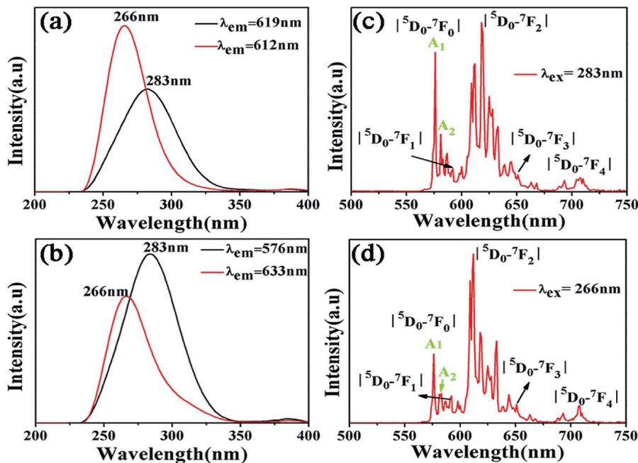
Fig. 3 (a) and (b) Excitation spectra under different monitoring wavelengths of  $\text{Ca}_5(\text{BO}_3)_3\text{F}:1\% \text{Eu}^{3+}$ ; (c) and (d) emission spectra of  $\text{Ca}_5(\text{BO}_3)_3\text{F}:1\% \text{Eu}^{3+}$  under 266 and 283 nm excitation.
