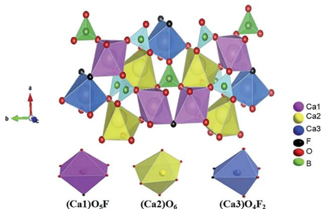
Fig. 2 Crystal structure of  $\text{Ca}_5(\text{BO}_3)_3\text{F}$  and the coordination environment of Ca1, Ca2, and Ca3.
