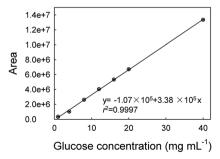
Fig. 8 Calibration curve of glucose measurement using a HPLC method.
