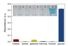
Fig. 6 UV-vis absorbance responses of the proposed biosensor to 5 mM maltose, 5 mM lactose, 5 mM galactose, 5 mM mannose, 5 mM fructose and 1 mM glucose (1 to 6). Inset: sample images of above reactions. Conditions: 0.75 mM FeCl<sub>3</sub>, 0.75 mM K<sub>3</sub>Fe(CN)<sub>6</sub> and 0.05 mg mL<sup>-1</sup> GOx in 50 mM MES (pH 3.0) at 25 °C.
