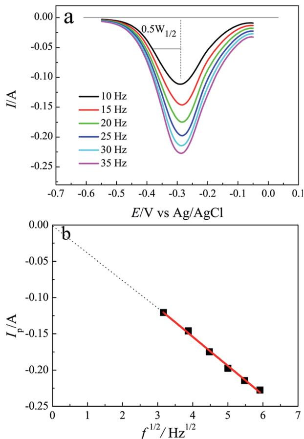
Fig. 2 (a) Square wave voltammograms of LiCl–KCl–PbCl<sub>2</sub> (0.60 wt%) melts on tungsten electrode (0.322 cm<sup>2</sup>) at different frequencies at 723 K; (b) peak current vs. square root of frequency. Pulse amplitude: 0.1 V; potential step: 0.005 V.
