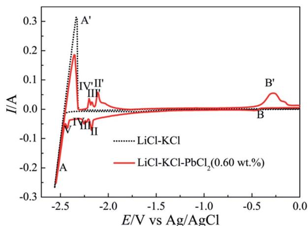
Fig. 1 Cyclic voltammograms of LiCl–KCl melts before (dotted curve) and after the addition of PbCl<sub>2</sub> (0.60 wt%) (red curve) at 723 K on tungsten electrode (0.322 cm<sup>2</sup>) at scan rate of 0.1 V s<sup>–1</sup>.
