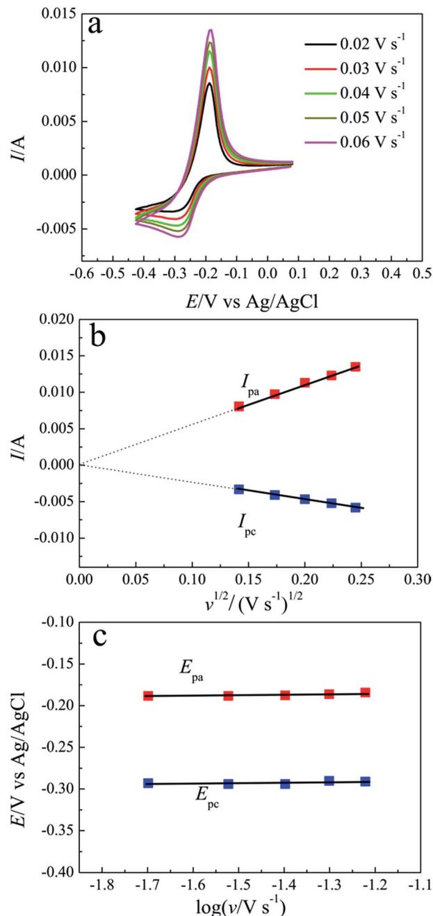
Fig. 3 (a) Cyclic voltammograms recorded in LiCl–KCl–PbCl<sub>2</sub> melts at 723 K on tungsten electrode (0.322 cm<sup>2</sup>) at different scan rates, (b) anodic and cathodic peak currents as a function of square root of scan rates and (c) anodic and cathodic peak potentials vs. logarithm of scan rates.
