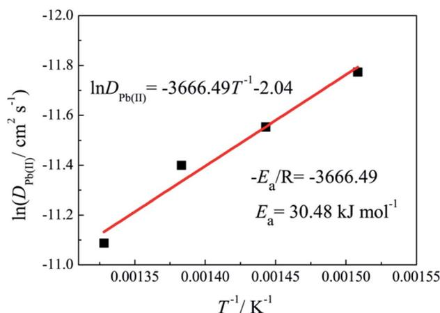
Fig. 4 The change of diffusion coefficients with temperatures.
