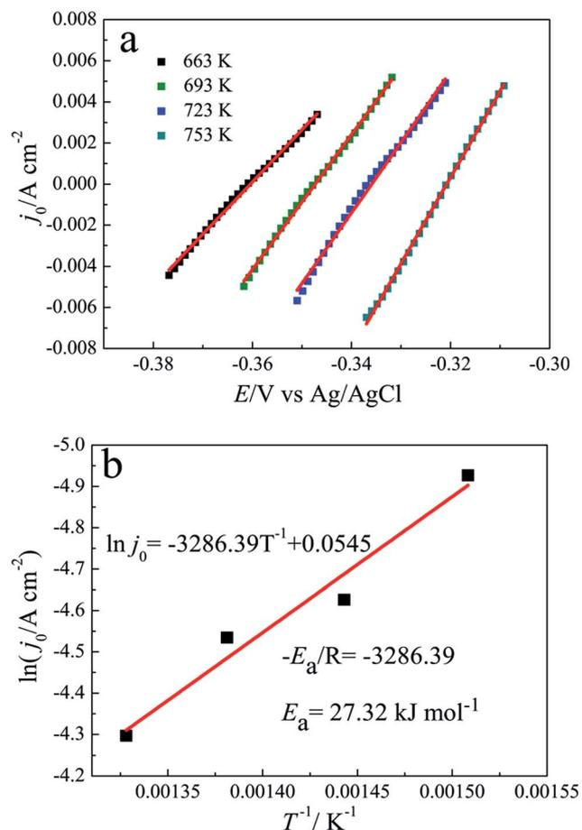
Fig. 5 (a) The linear polarization of LiCl–KCl–PbCl<sub>2</sub> (0.60 wt%) melts on tungsten electrode (0.322 cm<sup>2</sup>) at different temperature at scan rate of 0.005 V s<sup>-1</sup> and (b) the relationship between the reciprocal of the temperatures and the logarithm of exchange current densities.
