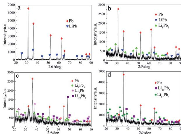
Fig. 10 XRD patterns of the samples obtained on a liquid Pb electrode in LiCl–KCl–PbCl<sub>2</sub> melts by galvanostatic electrolysis at 1.0 A for (a) 4 h, (b) 6 h, (c) 7 h and (d) 9 h at 723 K.
