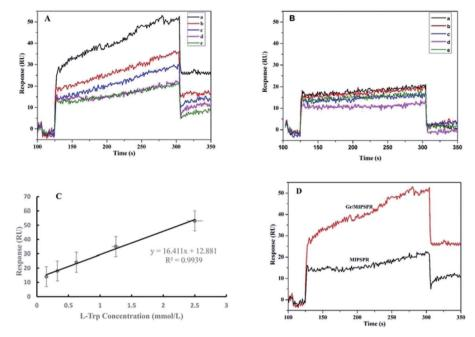
Fig. 3 SPR signals to different concentrations of (A)  $_{\rm L}$ -Trp and (B)  $_{\rm D}$ -Trp (a–e): 2.50, 1.25, 0.625, 0.325 and 0.150 mmol  $_{\rm L}^{-1}$ ; (C) the calibration curve for  $_{\rm L}$ -Trp on Gr/MIPSPR sensor; (D) SPR signals to 2.5 mmol  $_{\rm L}^{-1}$   $_{\rm L}$ -Trp on Gr/MIP-coated sensor and MIP-coated sensor. All SPR measurements were performed in phosphate-buffered saline with Tween (pH 8.0) at a flow rate of 20  $_{\rm L}$ L min $_{\rm L}^{-1}$ .
