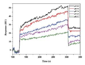
Fig. 2 Effect of pH on SPR signal (in the presence of 2.5 mmol  $L^{-1}L$ -Trp).
