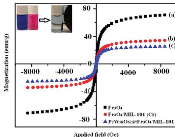
Fig. 7 Magnetic hysteresis loop of (a)  $Fe_3O_4$ , (b)  $Fe_3O_4/MIL-101$  (Cr), and (c)  $P_2W_{18}O_{62}@Fe_3O_4/MIL-101$  (Cr) at room temperature. The inset shows the behavior of the nanohybrid under an external magnetic field.
