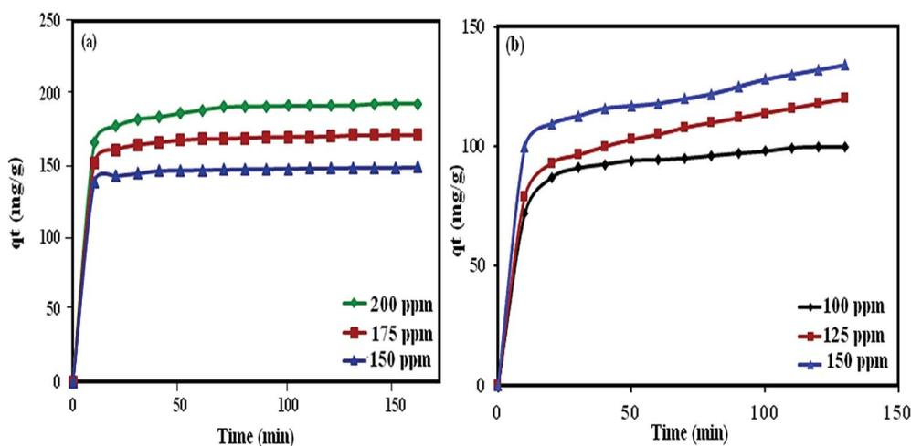
**Fig. 13** Effect of contact time and initial dye concentration on the adsorption process onto the P<sub>2</sub>W<sub>18</sub>O<sub>62</sub>@Fe<sub>3</sub>O<sub>4</sub>/MIL-101 (Cr) adsorbent.
