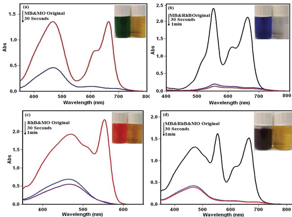
Fig. 12 Selective adsorption ability of P<sub>2</sub>W<sub>18</sub>O<sub>62</sub>@Fe<sub>3</sub>O<sub>4</sub>/MIL-101 (Cr) toward mixed dyes solution of (a) MB&MO, (b) MB&RhB, (c) RhB&MO, (d) MB&RhB&MO. Conditions: C<sub>0</sub> (MB) = C<sub>0</sub> (RhB) = C<sub>0</sub> (MO) = 25 mg L<sup>-1</sup>, and adsorbent dose = 30 mg/30 mL.
