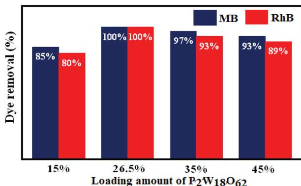
Fig. 10 Effects of different loading amounts of P<sub>2</sub>W<sub>18</sub>O<sub>62</sub> in MIL-101 (Cr) on the removal of MB and RhB dyes.
