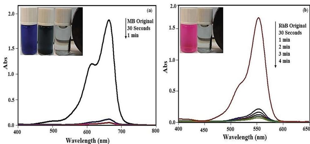
Fig. 8 UV-Vis spectral changes of dyes aqueous solutions with  $P_2W_{18}O_{62}@Fe_3O_4/MIL-101(Cr)$  at different time intervals: (a) MB dye, (b) RhB dye. [Dye] =  $25\text{ mg L}^{-1}$ , adsorbent:  $30\text{ mg}$  at  $25\text{ }^\circ\text{C}$ .
