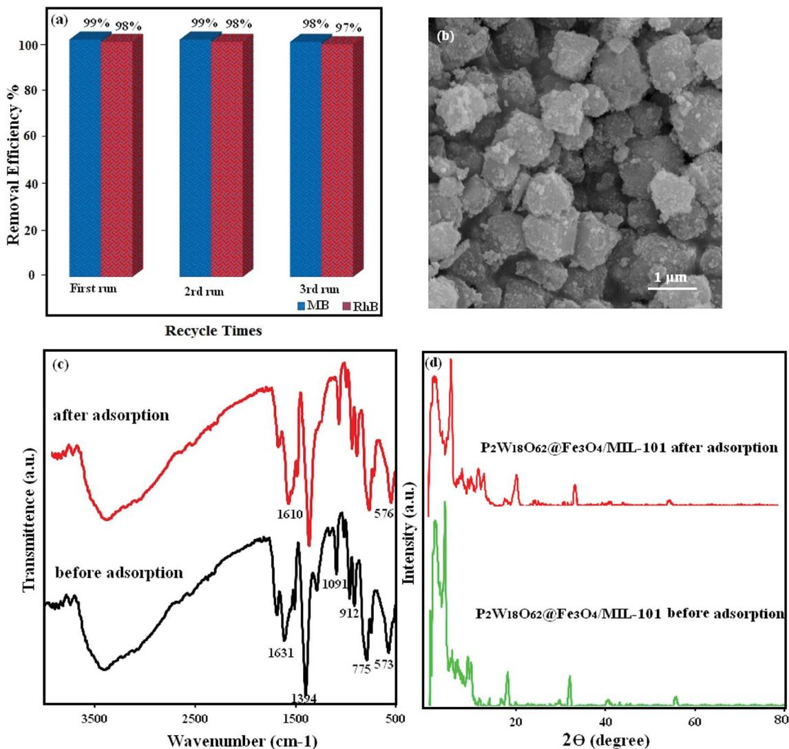
Fig. 15 (a) Recyclability of the  $P_2W_{18}O_{62}@Fe_3O_4/MIL-101$  (Cr) hybrid nanomaterial in the removal of MB dye, (b) SEM images, (c) FT-IR spectrum, and (d) XRD pattern of the fresh and recovered nanohybrid after three runs.
