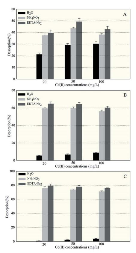
Fig. 2 The percentage of Cd(II) desorbed from Cd(II)-loaded biomass of *Cupriavidus necator* GX\_5 (A), *Sphingomonas* sp. GX\_15 (B), and *Curtobacterium* sp. GX\_31 (C), after treatment with ddH<sub>2</sub>O, 1.0 mol l<sup>-1</sup> of NH<sub>4</sub>NO<sub>3</sub>, and 0.1 mol l<sup>-1</sup> of EDTA-Na<sub>2</sub>, under 20, 50, and 100 mg l<sup>-1</sup> initial Cd(II) concentrations.
