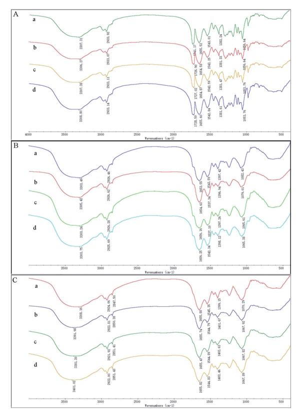
Fig. 6 FTIR images of Cupriavidus necator GX\_5 (A), Sphingomonas sp. GX\_15 (B), and Curtobacterium sp. GX\_31 (C) under different initial Cd(II) concentrations ((a) 0 mg l<sup>-1</sup> of Cd(II); (b) 20 mg l<sup>-1</sup> of Cd(II); (c) 50 mg l<sup>-1</sup> of Cd(II); and (d) 100 mg l<sup>-1</sup> of Cd(III).
