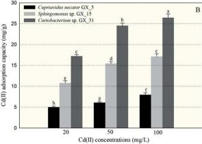
Fig. 1 The removal efficiency of Cd(II) (A) and adsorption capacity of Cd(II) (B) by Cupriavidus necator GX\_5, Sphingomonas sp. GX\_15, and Curtobacterium sp. GX\_31 under 20, 50, and 100 mg  $l^{-1}$  of initial Cd(II) concentrations.
