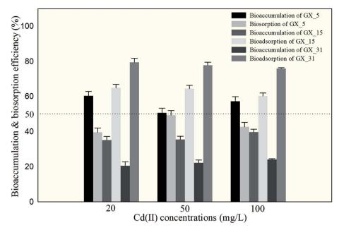
Fig. 3 Extracellular adsorption (biosorption) and intracellular accumulation (bioaccumulation) by *Cupriavidus necator* GX\_5, *Sphingomonas* sp. GX\_15, and *Curtobacterium* sp. GX\_31 under 20, 50, and 100 mg  $|^{-1}$  initial Cd(||) concentrations.
