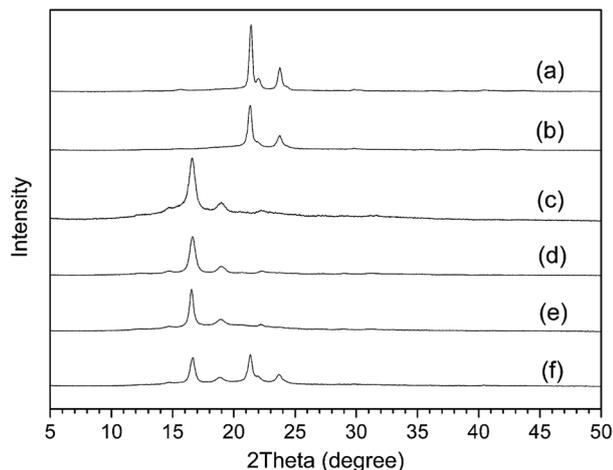
Fig. 14 X-ray diffraction pattern of synthetic polymers: (a) linear PCL, (b) 4sPCL, (c) linear PLLA, (d) 4sPLLA, (e) 4sPCL-*b*-PLLA, (f) PCL<sub>2</sub>PLLA<sub>2</sub>.
