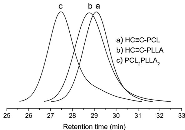
Fig. 11 GPC traces of (a) HC≡C-PCL, (b) HC≡C-PLLA and (c) PCL<sub>2</sub>PLLA<sub>2</sub>.
