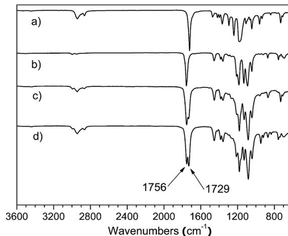
**Fig. 5** FT-IR spectra of star-shaped copolymers: (a) 4sPCL, (b) 4sPLLA, (c) 4sPCL-*b*-PLLA, (d) PCL<sub>2</sub>PLLA<sub>2</sub>.
