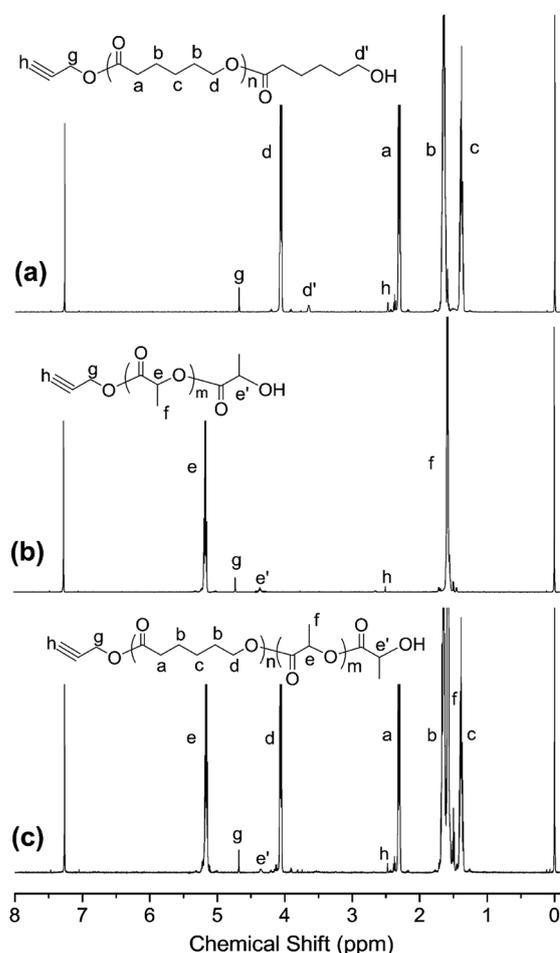
Fig. 4 <sup>1</sup>H-NMR spectra of (a) HC≡C-PCL, (b) HC≡C-PLLA and (c) HC≡C-PCL-*b*-PLLA.
