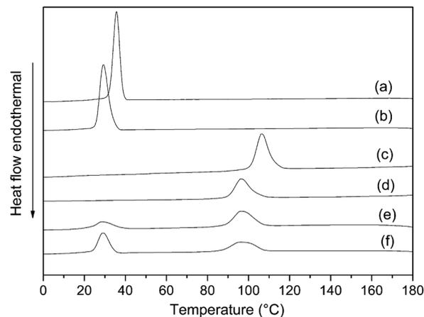
Fig. 12 DSC cooling curves of synthetic polymers: (a) linear PCL, (b) 4sPCL, (c) linear PLLA, (d) 4sPLLA, (e) 4sPCL-*b*-PLLA, (f) PCL<sub>2</sub>PLLA<sub>2</sub>.
