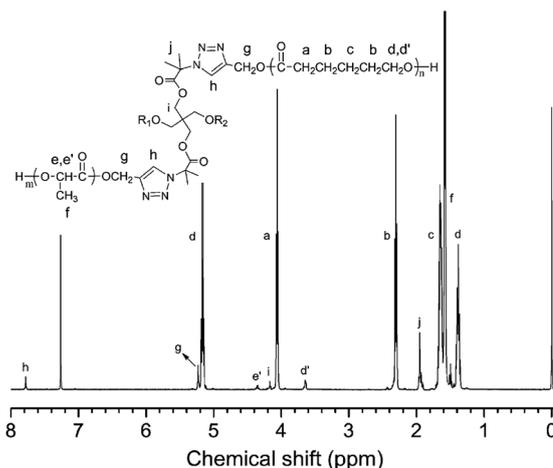
Fig. 10  $^1\text{H}$ -NMR spectra of the miktoarm star copolymer PCL<sub>2</sub>PLLA<sub>2</sub>.
