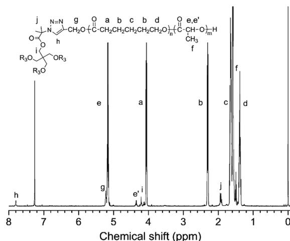
Fig. 8 <sup>1</sup>H-NMR spectra of the star-block copolymer 4sPCL-*b*-PLLA.
