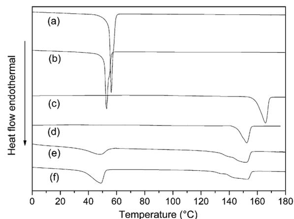
Fig. 13 Secondary heating DSC curve of synthetic polymers: (a) linear PCL, (b) 4sPCL, (c) linear PLLA, (d) 4sPLLA, (e) 4sPCL-*b*-PLLA, (f) PCL<sub>2</sub>PLLA<sub>2</sub>.
