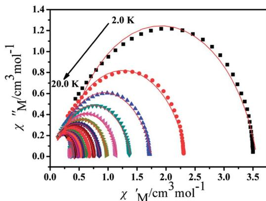
Fig. 11 Cole-Cole plots for  $\text{CH}_3\text{O}-2$  from 2.0 K to 20.0 K using the ac susceptibility data. The solid lines are the best fits for the generalized Debye model between 2.0 K and 20.0 K.
