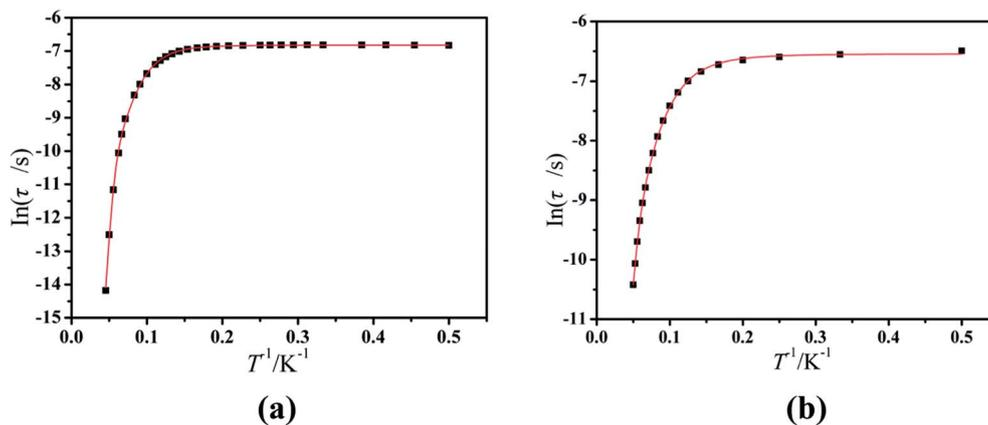
Fig. 12 Magnetization relaxation time ( $\ln(\tau)$ ) versus  $T^{-1}$  plots under a zero dc field for Cl-1 (a) and  $\text{CH}_3\text{O-2}$  (b). The solid red line represents the best fitting to the multiple relaxation processes (eqn (1), see text for parameters).
