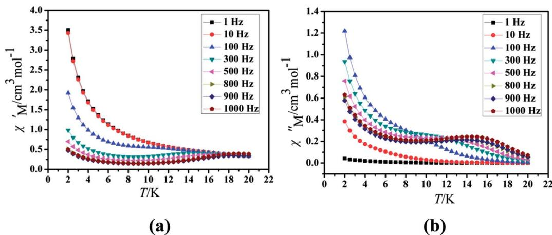
Fig. 7 Temperature dependence of the in-phase ( $\chi'$ , a) and out-of-phase ( $\chi''$ , b), respectively, of the ac susceptibility for CH<sub>3</sub>O-2 under the zero-dc field.
