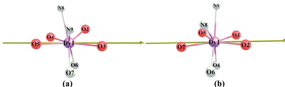
Fig. 13 Direction of the *ab initio* magnetic easy axis of the ground  $\text{KD}_s$  of the compounds (only the central Dy(III) and first sphere are shown for the sake of clarity, the equatorial atoms are shaded).
