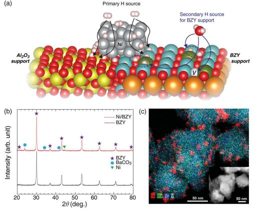
Fig. 1 (a) Schematic illustration of different hydrogenation processes occurring on Ni/BZY (right) and Ni/Al $_2$ O $_3$  (left) surfaces. (b) XRD patterns of as-prepared BZY support and the Ni/BZY catalyst. (c) TEM and EDS mapping images of as-prepared Ni/BZY, with Ni, Ba, Zr, and Y elements indicated by red, green, blue, and cyan colors, respectively.
