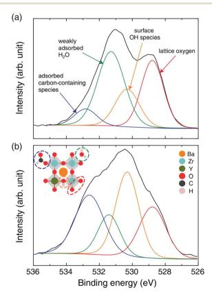
Fig. 6 O 1s core level XPS spectra of Ni/BZY (a) before and (b) after methanation. Red, yellow, green, and blue lines correspond to lattice oxygen, surface OH species, weakly adsorbed H<sub>2</sub>O, and adsorbed carbon-containing species (contaminant, BaCO<sub>3</sub> and formate), respectively
