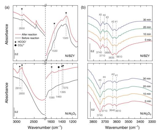
Fig. 4 In situ FT-IR spectra of species adsorbed on Ni/BZY and Ni/Al<sub>2</sub>O<sub>3</sub> during CO<sub>2</sub> methanation at 400 °C. (a) Analysis of formate (star) and carbonate (filled circle) species before/after CO<sub>2</sub> methanation. (b) Time-dependent analysis of OH groups contained in the flowing reactant gases at 400 °C. Red, yellow, green, and blue lines correspond to time steps of 0, 10, 20, and 30 min, respectively.
