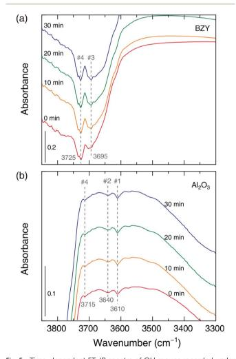
Fig. 5 Time-dependent FT-IR spectra of OH groups recorded under the conditions of reactant gas flow at 400 °C [(a): BZY, (b): Al<sub>2</sub>O<sub>3</sub>]. Red, yellow, green, and blue lines correspond to times of 0, 10, 20, and 30 min, respectively.
