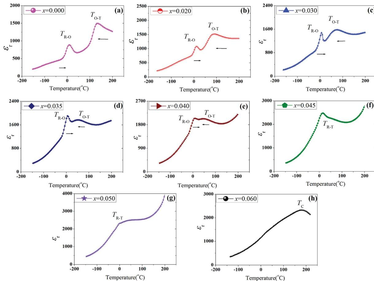
Fig. 2  $\epsilon_r$ - $T$  curves of  $(1-x)\text{K}_{0.44}\text{Na}_{0.56}\text{Nb}_{0.96}\text{Sb}_{0.04}\text{O}_3-x\text{Bi}_{0.45}\text{La}_{0.05}\text{Na}_{0.5}\text{ZrO}_3$  ceramics in temperature range of  $-150$ – $200$  °C.
