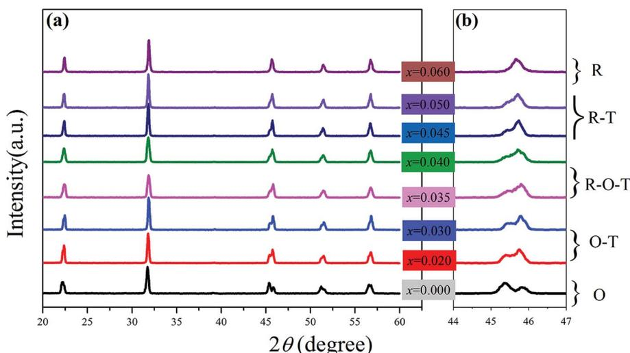
Fig. 1 XRD patterns of the  $(1-x)\text{K}_{0.44}\text{Na}_{0.56}\text{Nb}_{0.96}\text{Sb}_{0.04}\text{O}_3-x\text{Bi}_{0.45}\text{La}_{0.05}\text{Na}_{0.5}\text{ZrO}_3$  ceramics in the  $2\theta$  range of (a)  $20$ – $60^\circ$ , (b)  $44$ – $47^\circ$ .
