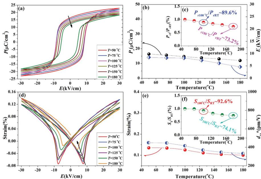
Fig. 10 Ferroelectric loops and bipolar electric field induced strain of  $0.96\text{K}_{0.44}\text{Na}_{0.56}\text{Nb}_{0.96}\text{Sb}_{0.04}\text{O}_3-0.04\text{Bi}_{0.45}\text{La}_{0.05}\text{Na}_{0.5}\text{ZrO}_3$  ceramics as a function of temperature from room temperature to  $180\text{ }^\circ\text{C}$ .
