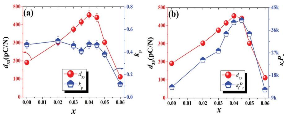
Fig. 8 (a) Piezoelectric ( $d_{33}$ ,  $k_p$ ) properties of  $(1-x)\text{K}_{0.44}\text{Na}_{0.56}\text{Nb}_{0.96}\text{Sb}_{0.04}\text{O}_3-x\text{Bi}_{0.45}\text{La}_{0.05}\text{Na}_{0.5}\text{ZrO}_3$  ceramics; (b)  $d_{33}$  and  $\epsilon_r P_r$  properties of  $(1-x)\text{K}_{0.44}\text{Na}_{0.56}\text{Nb}_{0.96}\text{Sb}_{0.04}\text{O}_3-x\text{Bi}_{0.45}\text{La}_{0.05}\text{Na}_{0.5}\text{ZrO}_3$  ceramics.
