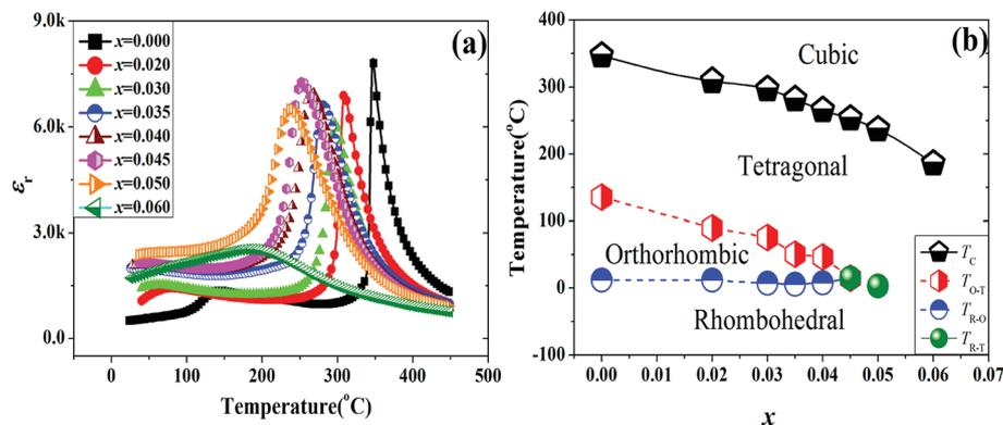
Fig. 3 (a)  $\epsilon_r$ - $T$  curves of  $(1-x)\text{K}_{0.44}\text{Na}_{0.56}\text{Nb}_{0.96}\text{Sb}_{0.04}\text{O}_3-x\text{Bi}_{0.45}\text{La}_{0.05}\text{Na}_{0.5}\text{ZrO}_3$  ceramics in temperature range of  $20$ – $450$  °C; (b) Phase diagrams of  $(1-x)\text{K}_{0.44}\text{Na}_{0.56}\text{Nb}_{0.96}\text{Sb}_{0.04}\text{O}_3-x\text{Bi}_{0.45}\text{La}_{0.05}\text{Na}_{0.5}\text{ZrO}_3$  ceramics.
