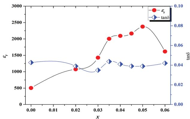
Fig. 6 Dielectric ( $\epsilon_r$ ,  $\tan \delta$ ) properties of  $(1-x)\text{K}_{0.44}\text{Na}_{0.56}\text{Nb}_{0.96}\text{Sb}_{0.04}\text{O}_3-x\text{Bi}_{0.45}\text{La}_{0.05}\text{Na}_{0.5}\text{ZrO}_3$  ceramics.
