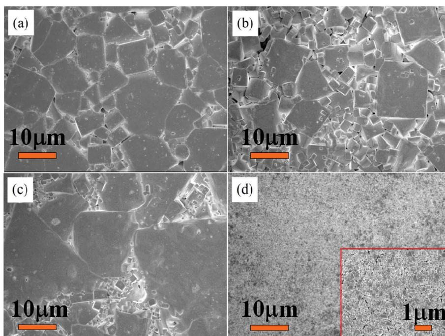
Fig. 4 FE-SEM surface images of  $(1-x)\text{K}_{0.44}\text{Na}_{0.56}\text{Nb}_{0.96}\text{Sb}_{0.04}\text{O}_3-x\text{Bi}_{0.45}\text{La}_{0.05}\text{Na}_{0.5}\text{ZrO}_3$  ceramics with (a)  $x = 0$ , (b)  $x = 0.020$ , (c)  $x = 0.040$ , (d)  $x = 0.060$ .
