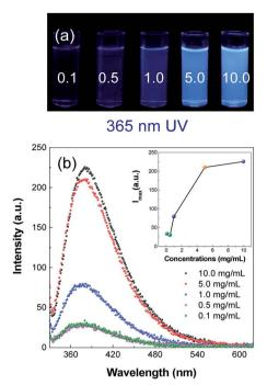
Fig. 2 (a) Photographs taken under 365 nm UV light and (b) fluorescence spectra of PASAS aqueous solutions with different concentrations.
