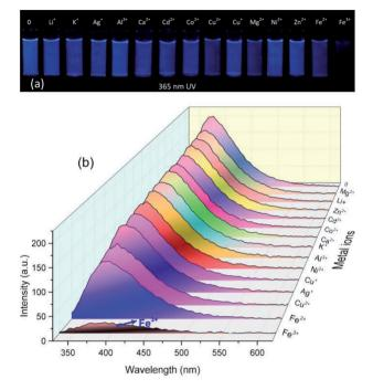
Fig. 4 (a) Photographs taken under 365 nm UV light and (b) fluorescence spectra of PASAS aqueous solution (5 mg mL $^{-1}$ ) in the presence of various metal ions (2  $\times$  10 $^{-3}$  mol L $^{-1}$ ).
