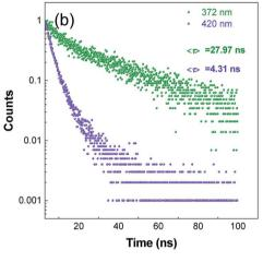
Fig. 1 (a) Fluorescence spectra of PASAS aqueous solution (10 mg  $\,\mathrm{mL}^{-1}$ ) with different excitation wavelengths. (b) The effect of excitation wavelength on fluorescence lifetime of PASAS aqueous solution (10 mg  $\,\mathrm{mL}^{-1}$ ).
