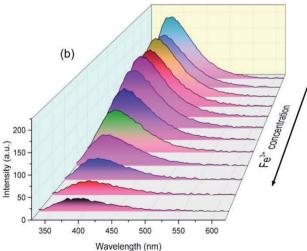
Fig. 5 (a) Photographs taken under 365 nm UV light and (b) fluorescence spectra of PASAS aqueous solution (5 mg  $\rm mL^{-1}$ ) on addition of different concentrations of Fe<sup>3+</sup>.
